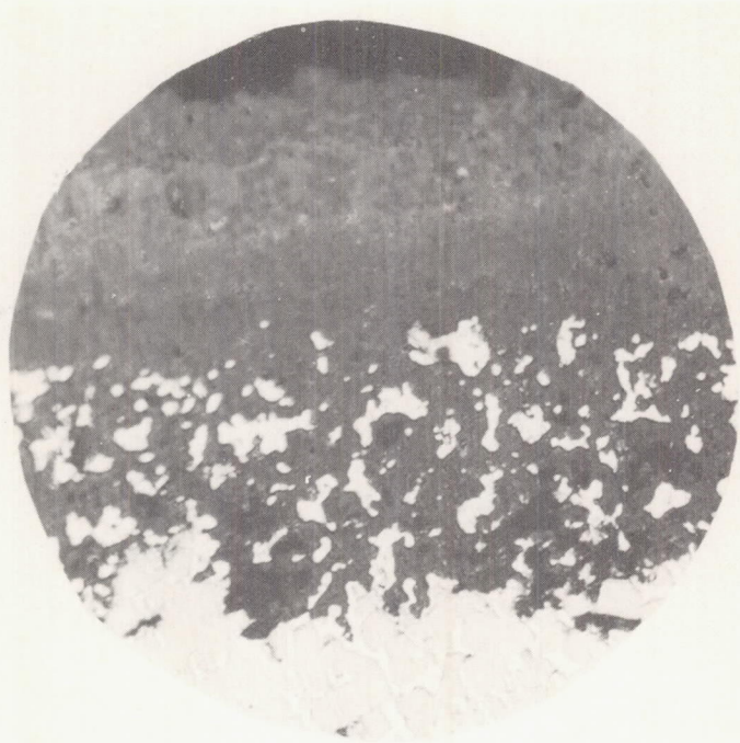
(g) Oxidized for 100 hours at 1600° F.
