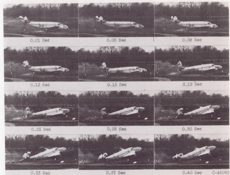
(b) Sequence pictures and accelerations of 16° crash of low-wing unpressurized transport. Impact speed, 109 mph.
