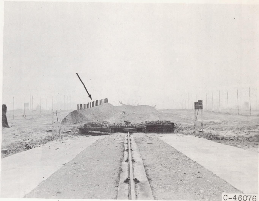
(c) Wing barrier used to produce groundloop crash.
