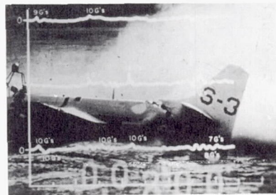
Figure 13. - Sequence pictures of cartwheel crash of FH-1 fighter airplane with superimposed acceleration graphs. Top curve, longitudinal; middle curve, normal; bottom curve, lateral.
