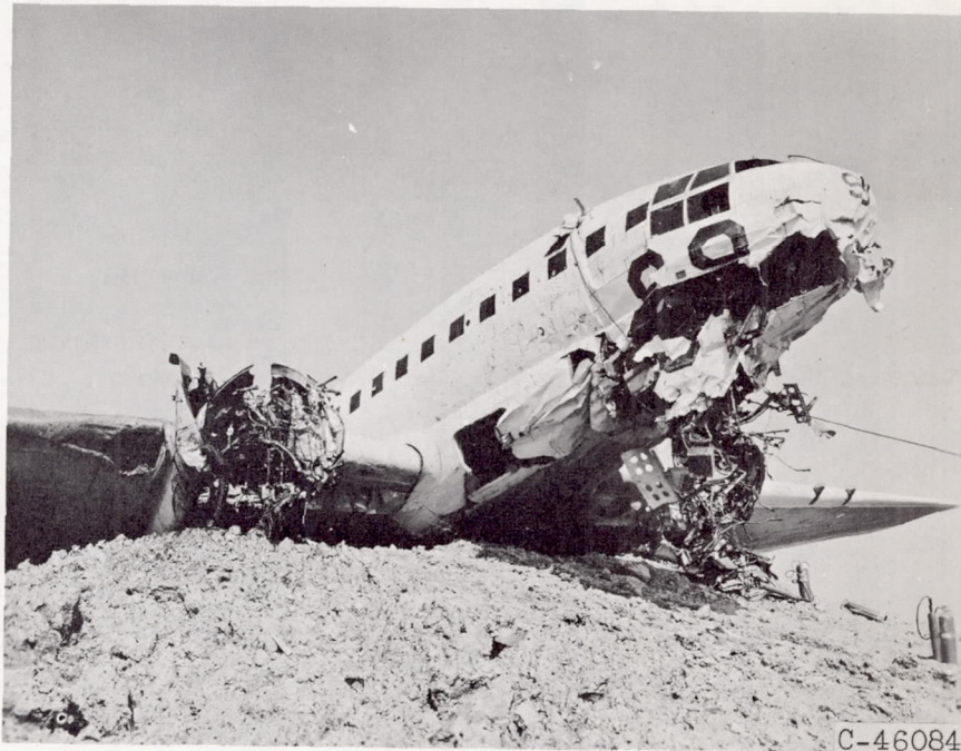
(c) Angle of impact, 29^{\circ} ; impact speed, 97 mph.
