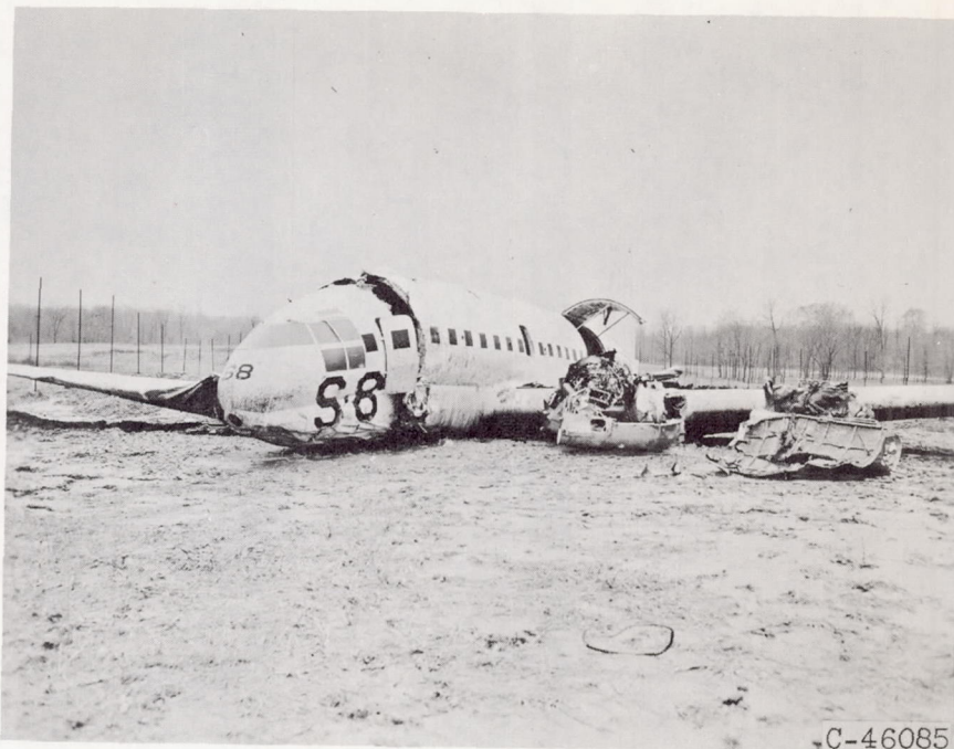
(b) Angle of impact, 15^{\circ} ; impact speed, 93 mph.
