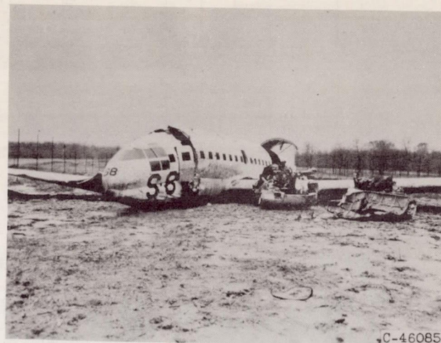
(b) Angle of impact, 15°; impact speed, 93 mph.
