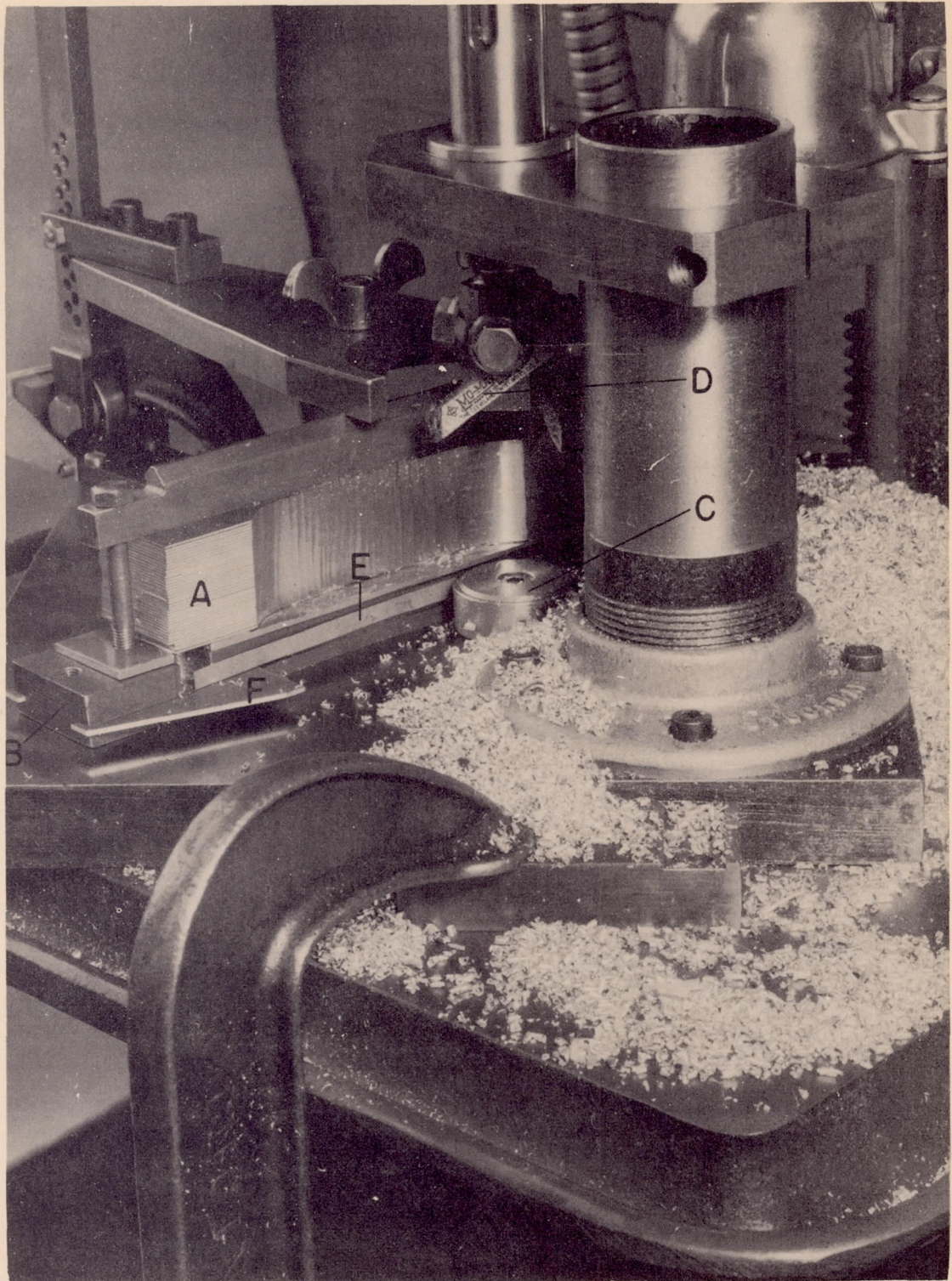
Figure 6.- Apparatus for machining reduced-section specimens.
