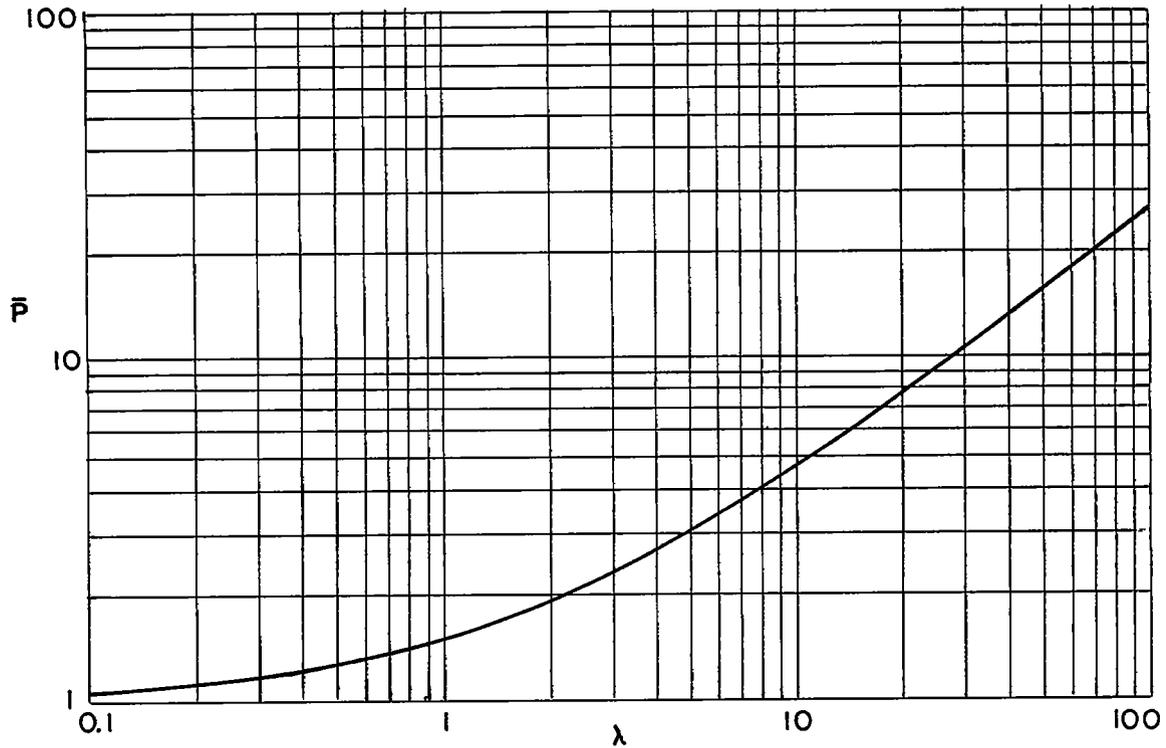
Figure 4.- Variation of the stringer stress concentration factor  $\bar{K}$
