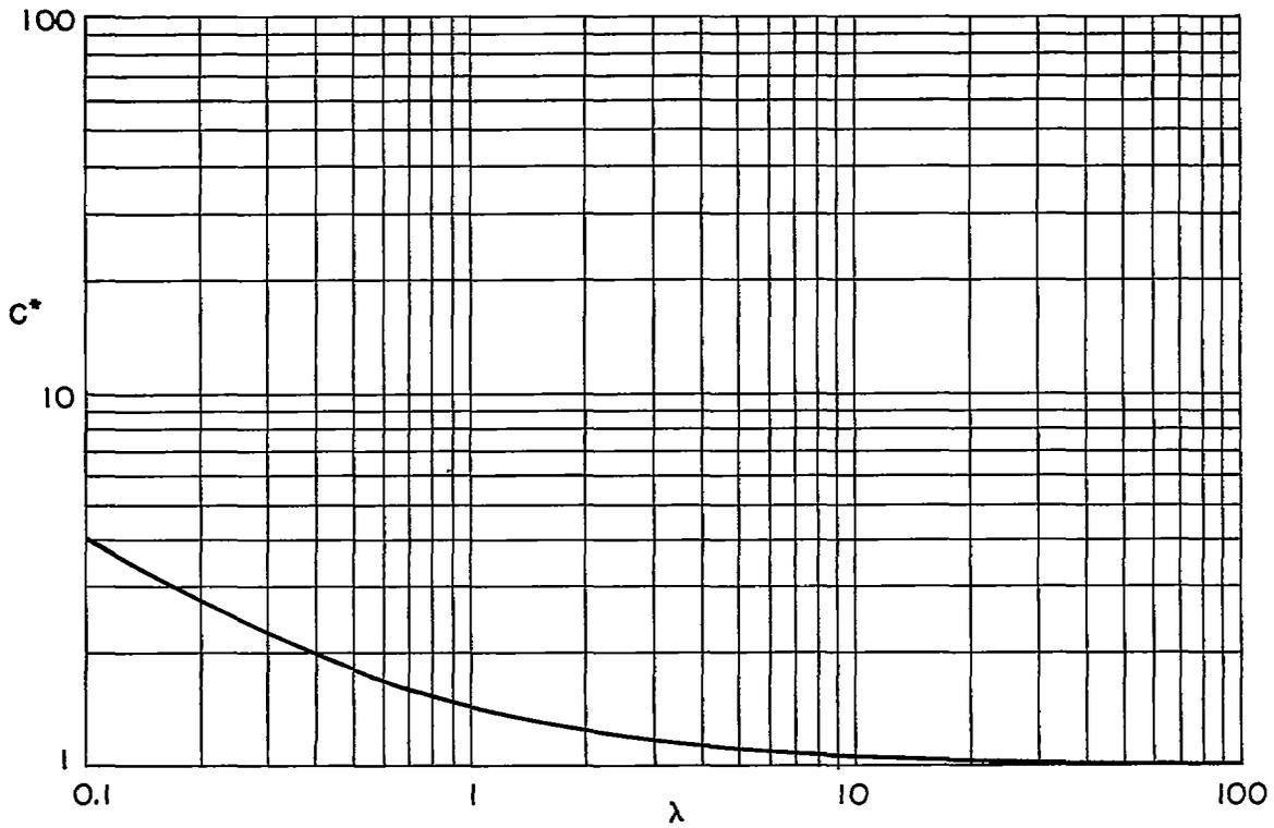
Figure 5.- Variation with  $\lambda$  of the ratio  $C^*$  of the stress concentration factors in a cracked sheet with and without a stringer for the case in which the stringer is broken.  $\lambda = \frac{2btE}{AE_{st}}$ .
