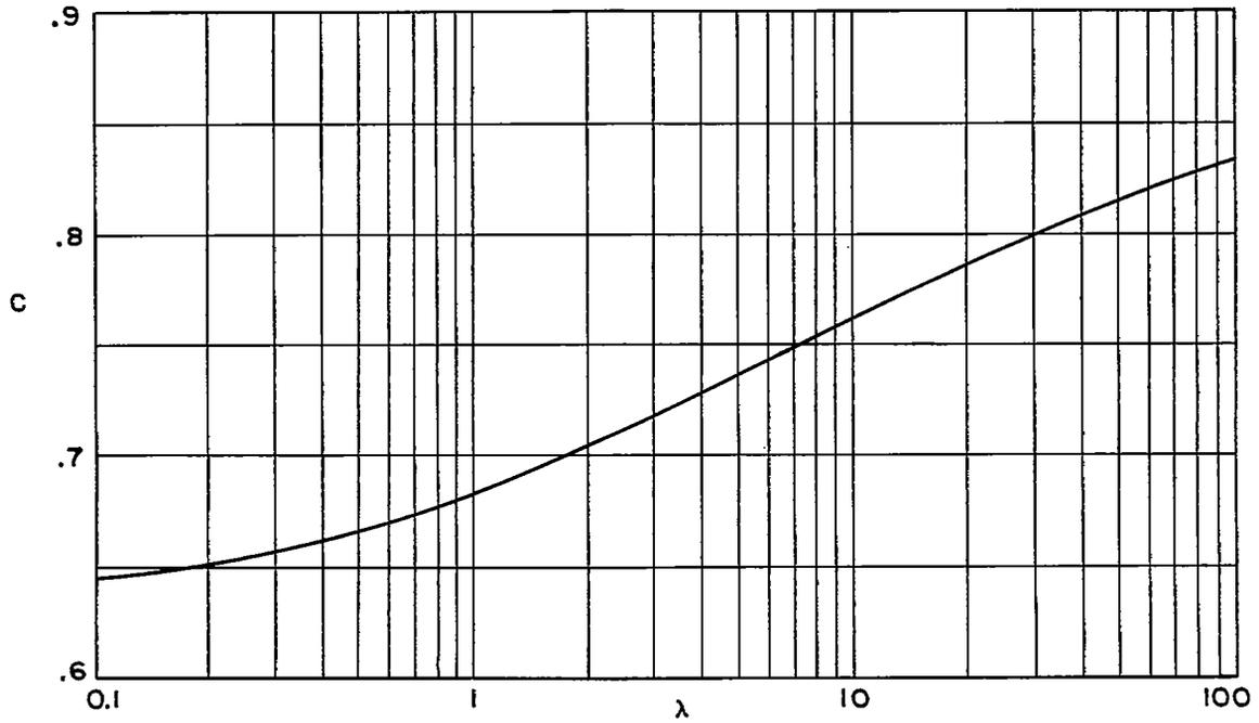
Figure 3.- Variation with  $\lambda$  of the ratio  $C$  of the stress concentration factors in a cracked sheet with and without a stringer for the case in which the stringer is intact.  $\lambda = \frac{2btE}{AE_{st}}$ .
