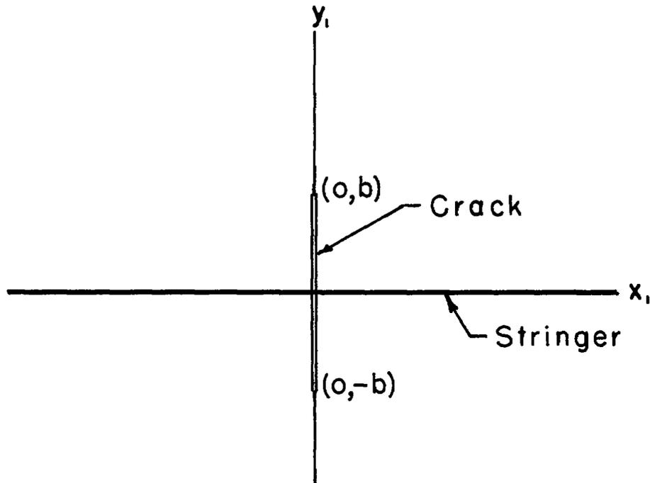
Figure 1.- Cracked sheet with a reinforcing stringer.
