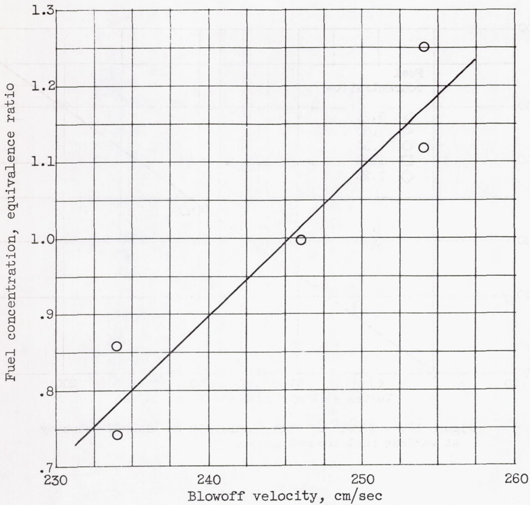
Figure 13. - Effect of equivalence ratio on blowoff velocity at constant vortex strength of 108 square centimeters per second.
