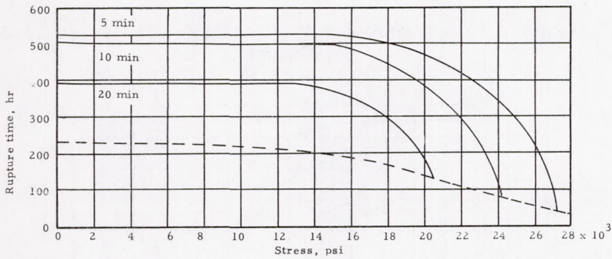
(e) Overheats to 1,800° F for HS-31 alloy. Stress at 1,500° F, 24,000 psi.
