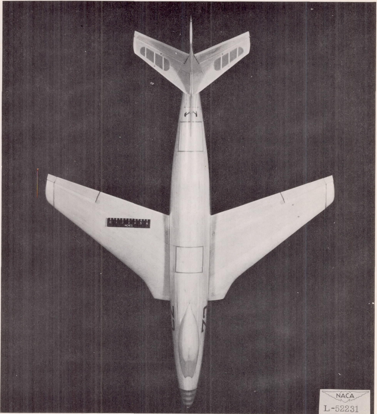
Figure 3.- Plan view of model with a 35° sweptback wing. Intake-duct fairings off.
