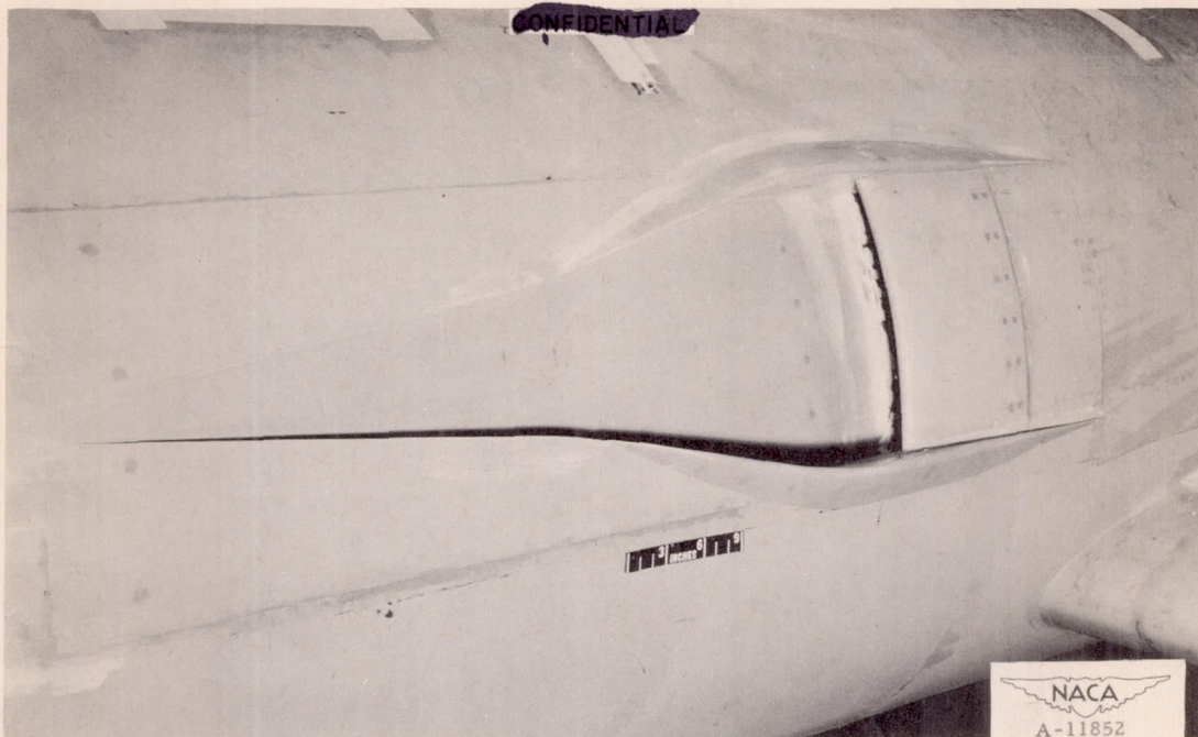
(a) 7^\circ ramp, standard divergence.
