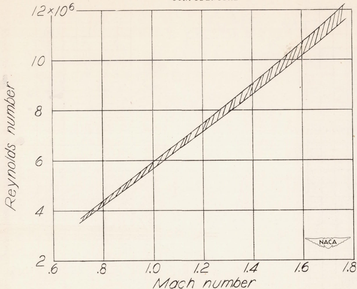
Figure 5.- Variation of Reynolds number with Mach number for the range of climatic conditions encountered.
