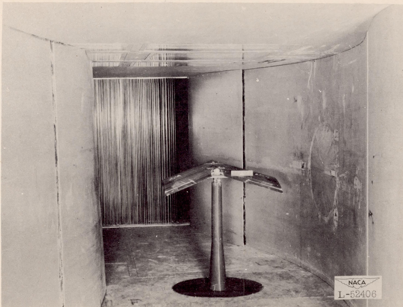
Figure 3.- The 45^{\circ} sweptback wing mounted in the curved-flow test section of the Langley stability tunnel. NACA 0012 airfoil section.
