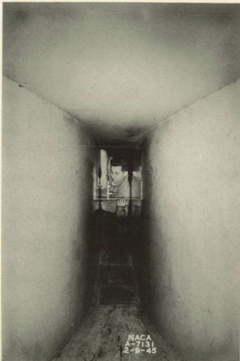
Figure 1.- Airfoil model mounted in the test section of the Ames 1 - by 3 1/2 foot high-speed wind tunnel.
