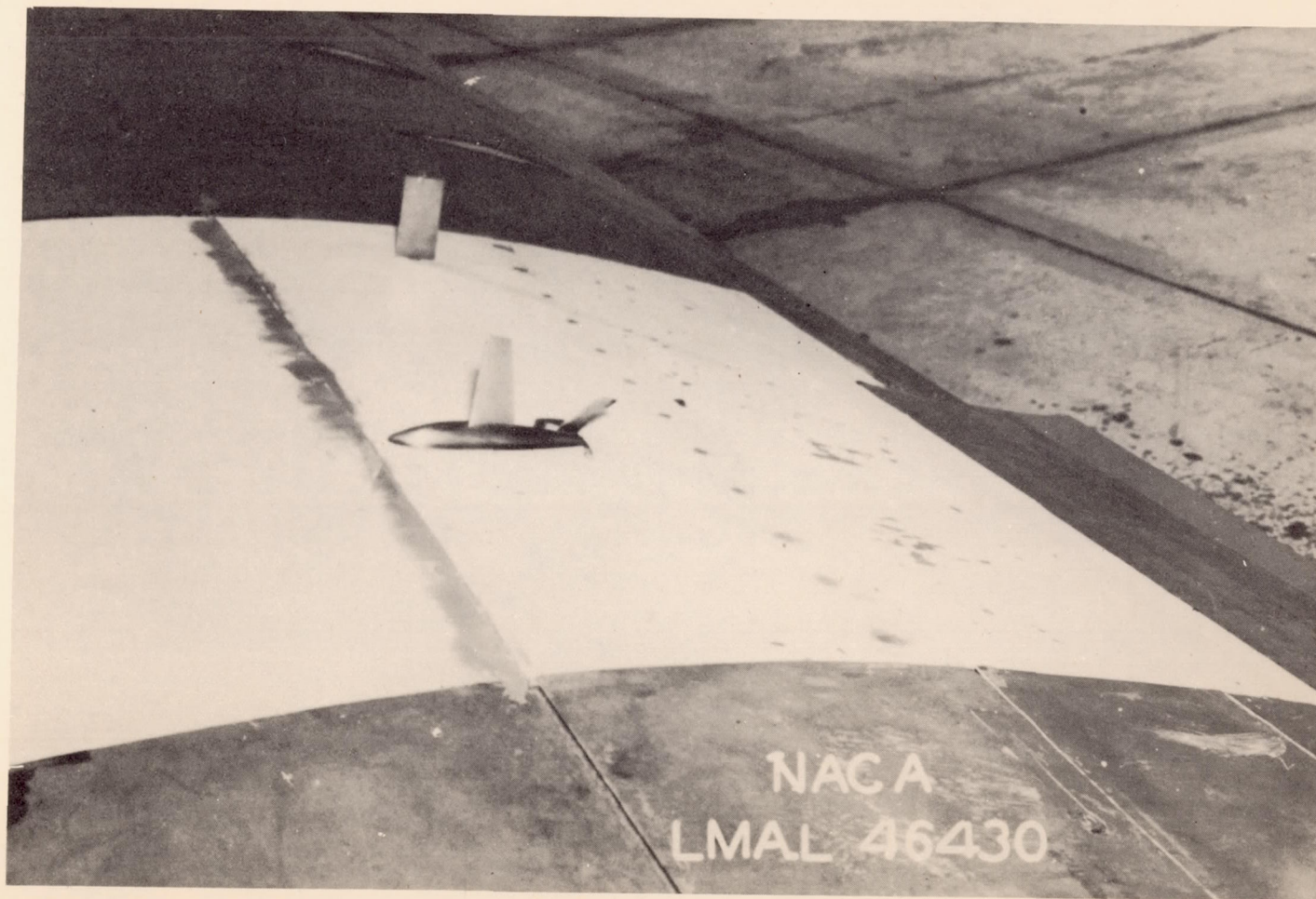
Figure 2.- Semispan airplane model mounted above wing of P-51D airplane.
