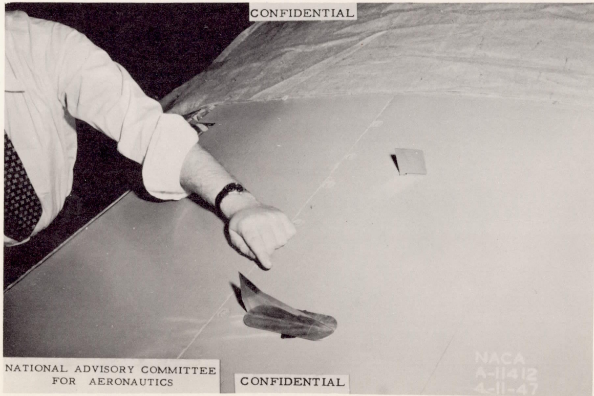
Figure 5.-- Wing-flow-method test station with low-aspect ratio wing-control model installed.
