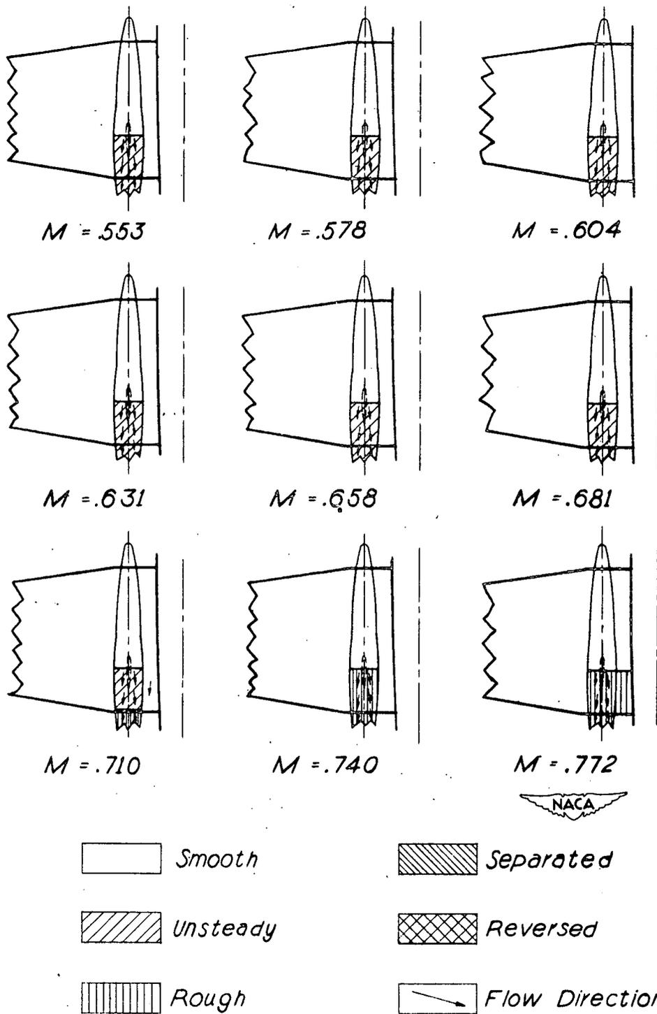
Figure 26.- Tuft studies of the lower surface of the store and the lower surface of the right wing of a wing-fuselage combination at various Mach numbers with the external store with a fan-shaped tail in place,  $\alpha = -.75^\circ$ ,  $\psi = 0^\circ$ ,  $\alpha_t = 0^\circ$ .
