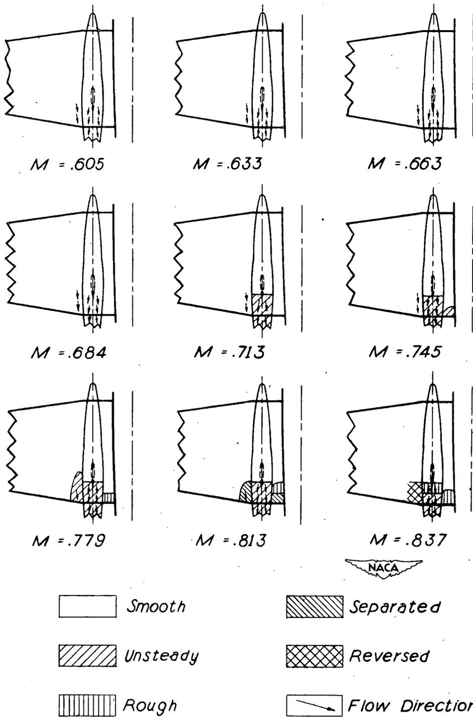
Figure 27.- Tuft studies of the lower surface of the store and the lower surface of the right wing of a wing-fuselage combination at various Mach numbers with the external store with a fan-shaped tail in place,  $\alpha = -.75^\circ$ ,  $\nu = 0^\circ$ ,  $\alpha_t = -2 \frac{1}{2}^\circ$ .
