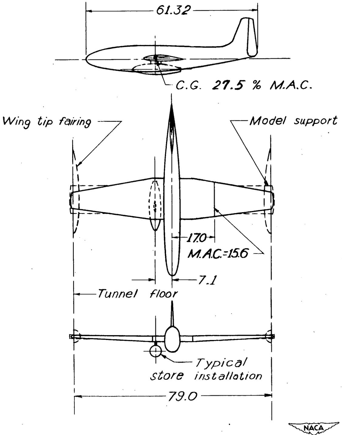
Figure 1.- Three-view drawing of the wing-fuselage combination mounted in the Langley high-speed 7-by 10-foot tunnel.
