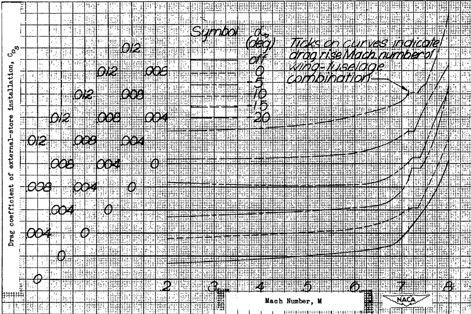
Figure 17.- Effect of the angular position of the auxiliary wing on the variation of the drag coefficient of the external-store installation with Mach number for the auxiliary wing arrangement mounted on the right wing of a wing-fuselage combination,  $\alpha = -0.75^\circ$ ,  $\psi = 0^\circ$ .
