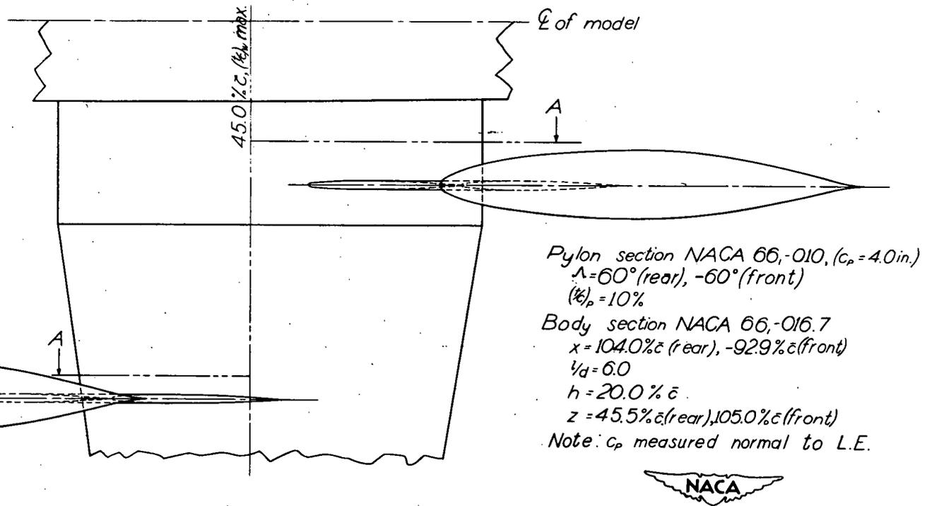
Figure 2. - Drawing of the tandem mounted arrangement as tested on the right wing of a wing-fuselage combination.
