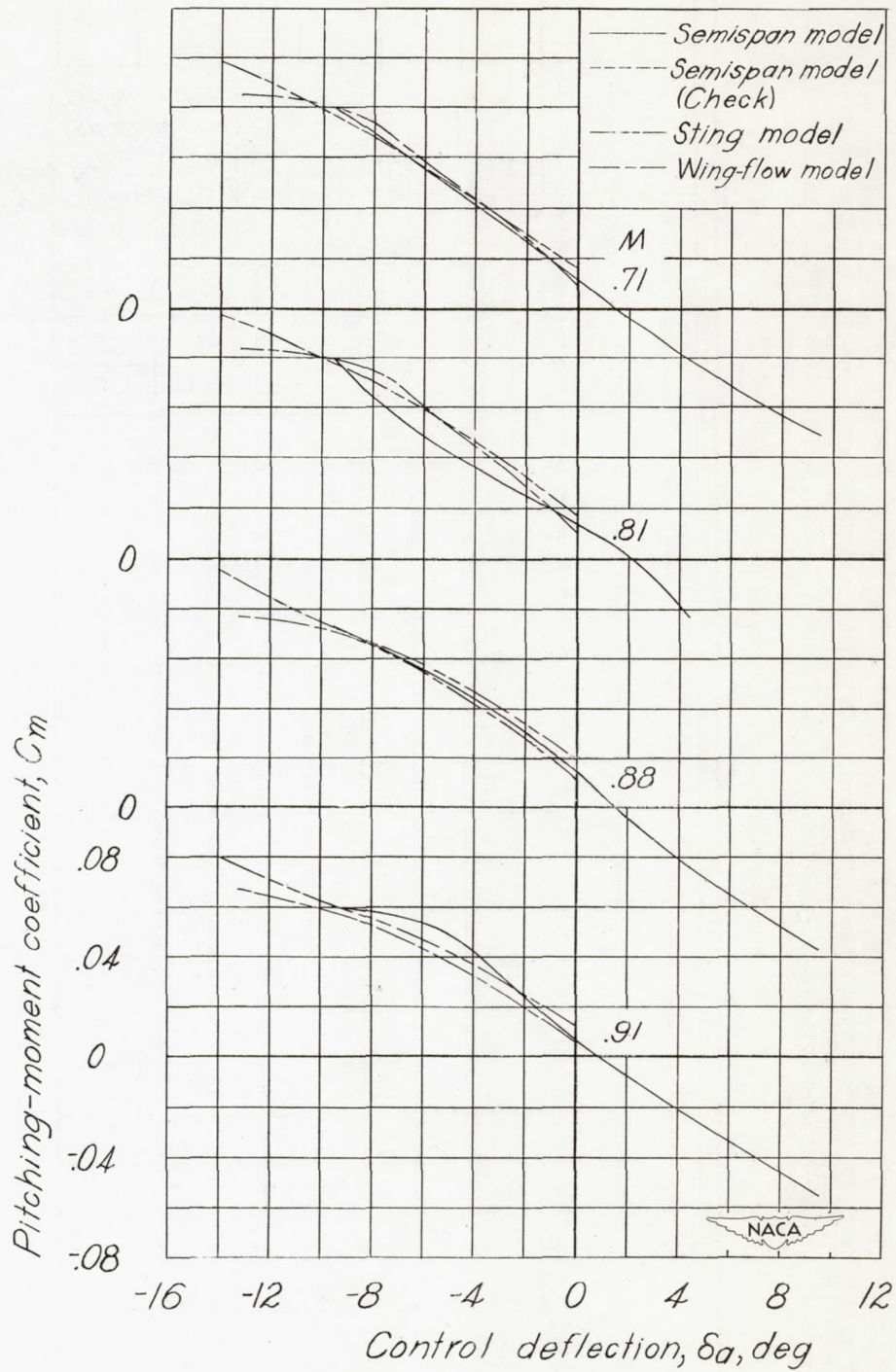
Figure 21.— A comparison of effectiveness for several Mach numbers as obtained by three different test methods on models of a tailless airplane. Vertical fins on; C_L = 0 .
