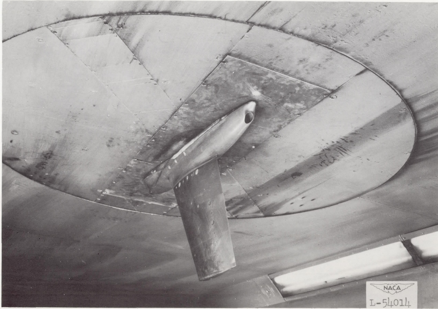
Figure 4.- The semispan model of a tailless airplane with vertical fin removed, mounted on the Langley 7- by 10-foot high-speed tunnel ceiling.
