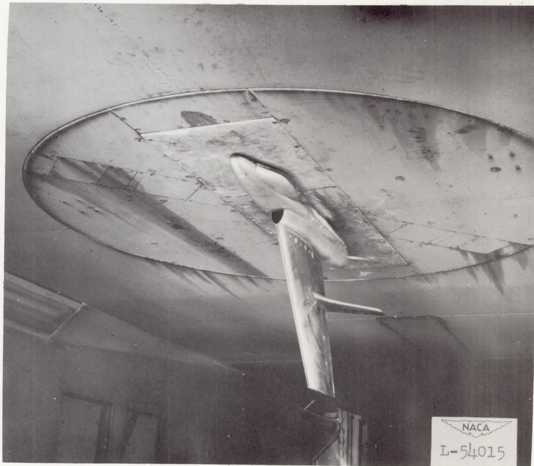
Figure 3.- The semispan model of a tailless airplane with vertical fin on, mounted on the Langley 7- by 10-foot high-speed tunnel ceiling.
