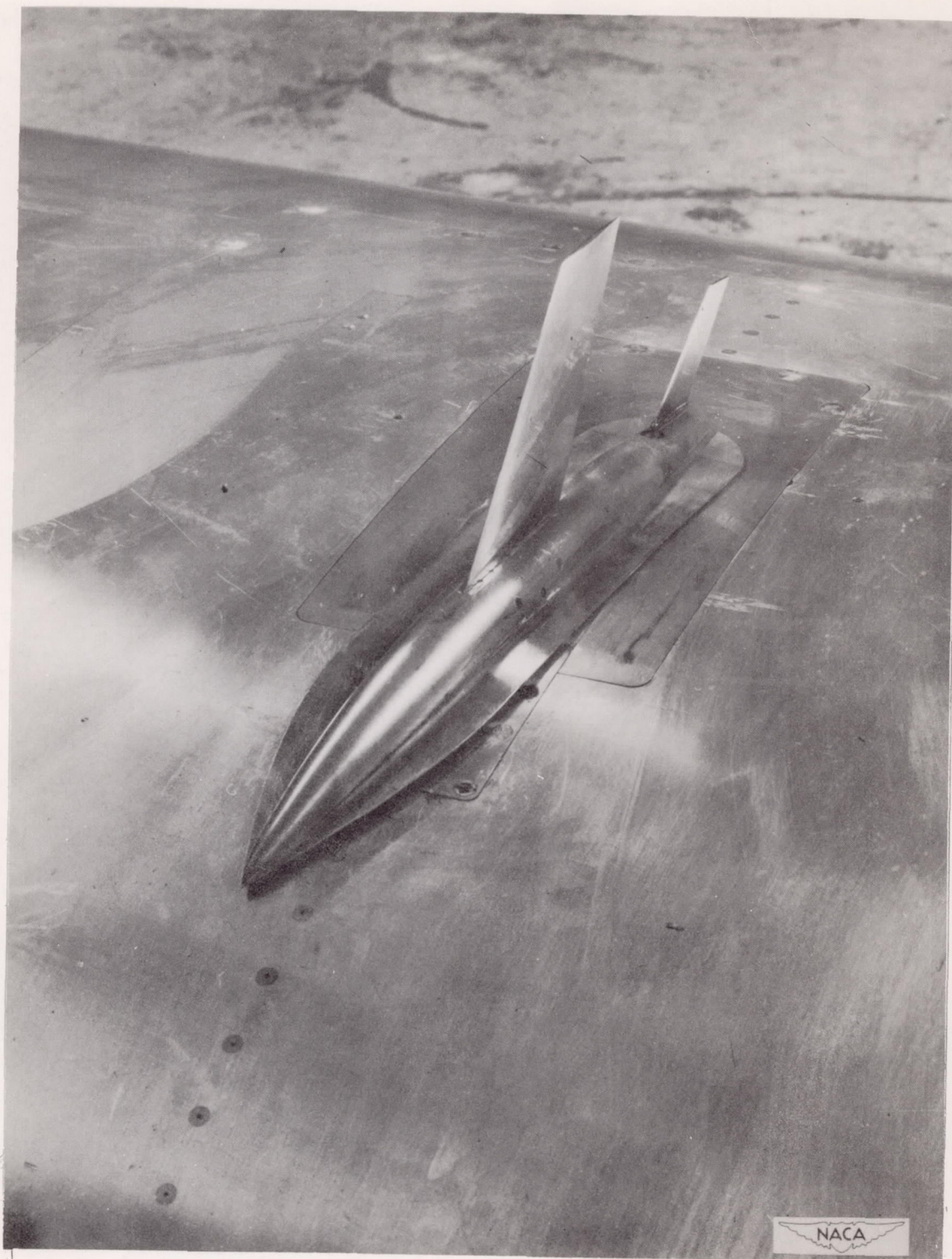
Figure 4.- Photograph of a model with 35^\circ sweptback wing, aspect ratio 4, taper ratio 0.6, and NACA 65A006 airfoil showing free-floating tail mounted in fuselage.
