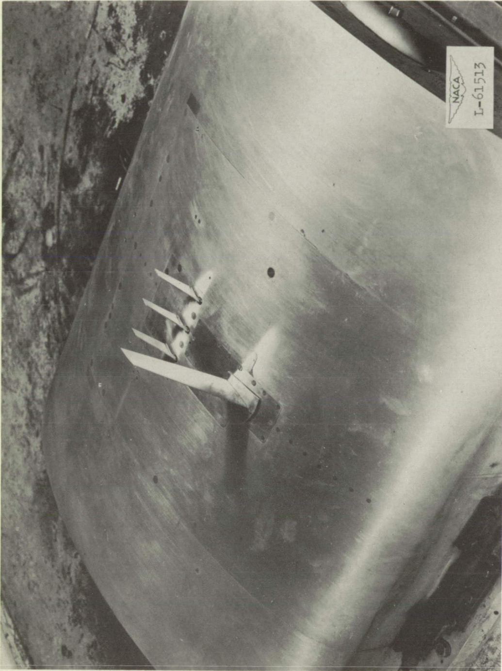
Figure 4.- Photograph of model with 35^\circ sweptback wing, aspect ratio 6, taper ratio 0.6, and NACA 65A006 airfoil.
