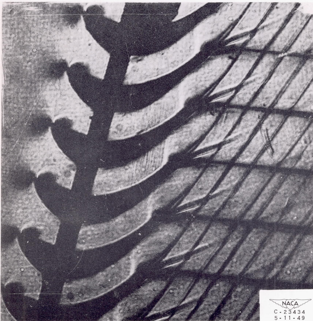
Figure 26. - Enlargement of schlieren photograph of flow through passages of 0.60-inch blades with schlieren knife edge parallel to inlet-flow direction. Pressure ratio p_4/p'_1 , 0.23.
