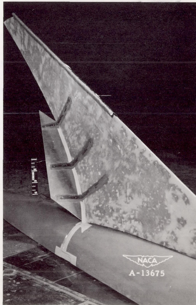
(e) Three-quarter-front view of the wing showing the leading- and trailing-edge flaps.
