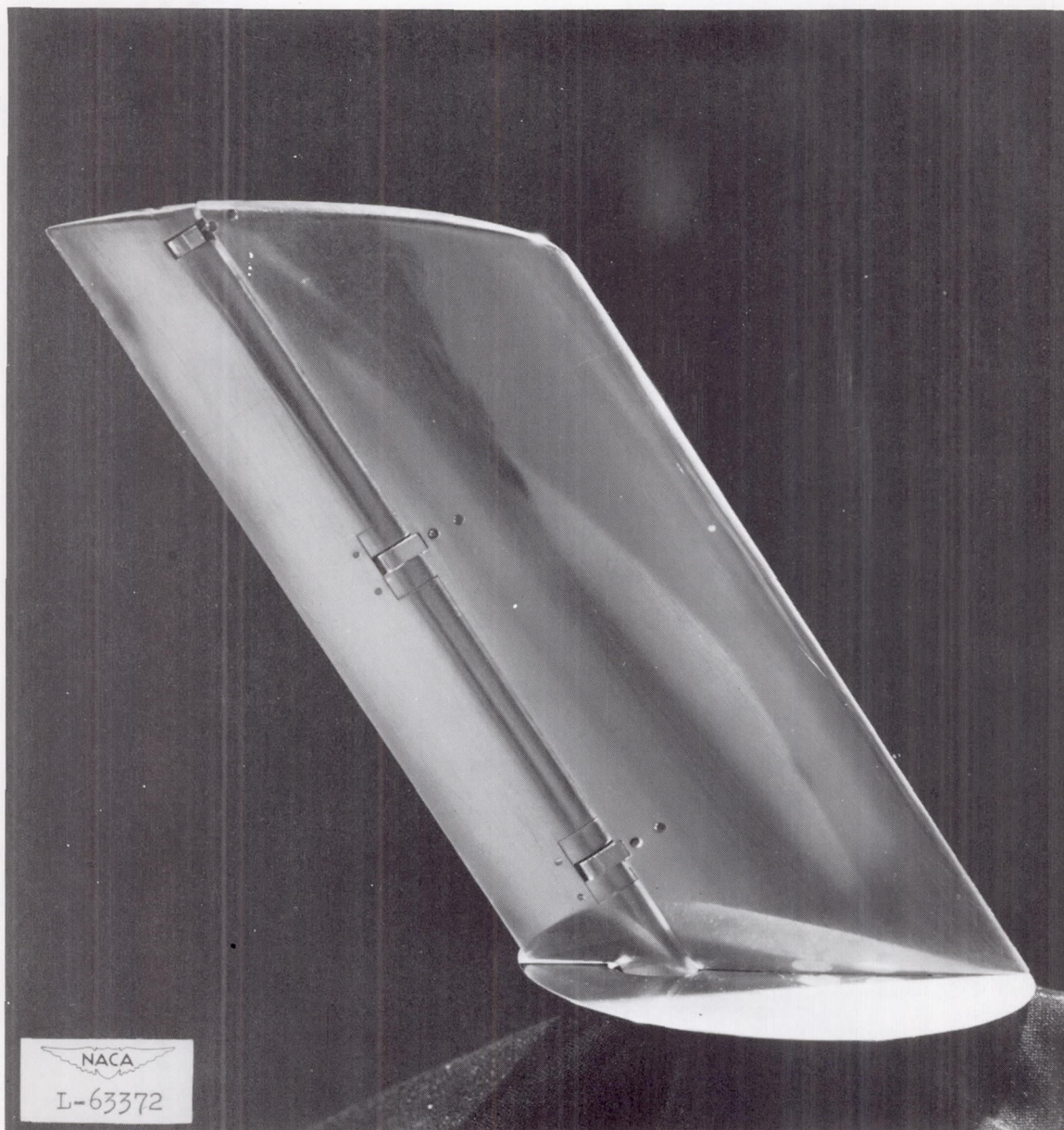
Figure 3.- Photograph of 35° sweptback NACA 65-009 model with \frac{1}{4} -chord overhang-balanced flap.
