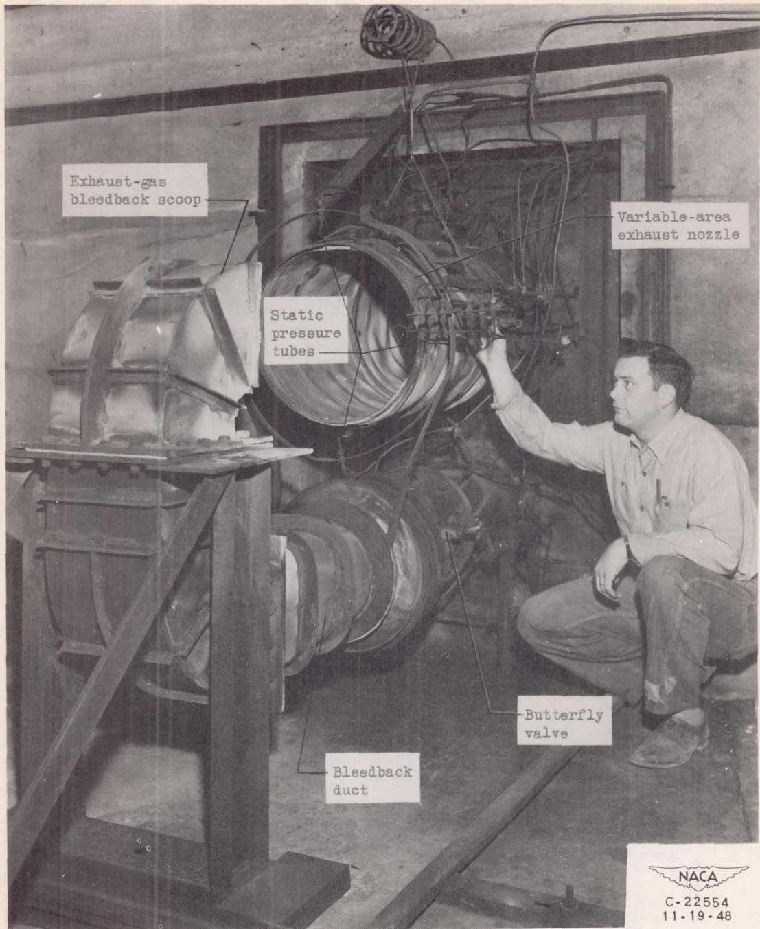
Figure 2. - View in muffler showing engine exhaust nozzle and exhaust-gas bleedback scoop.
