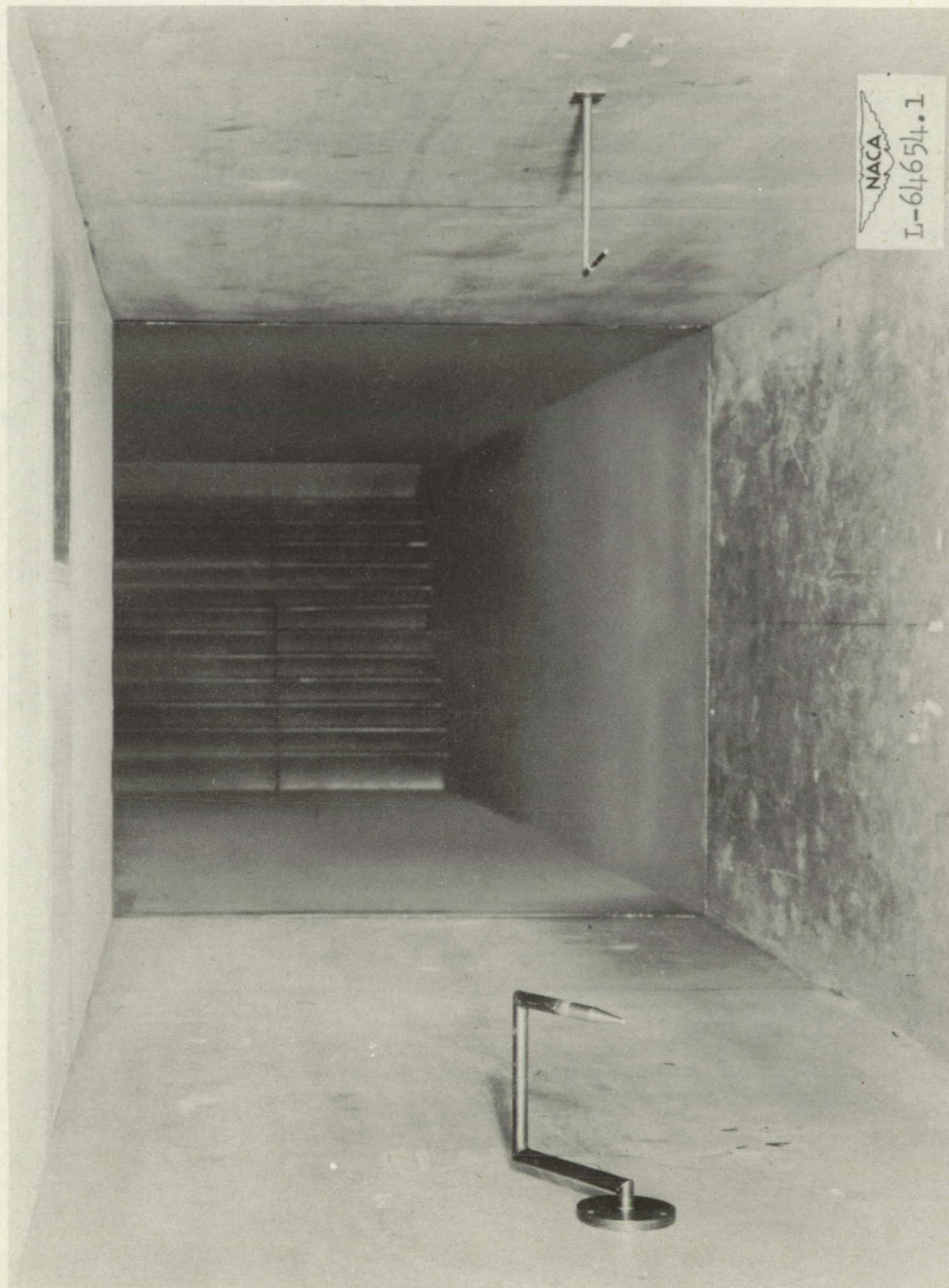
Figure 6.- View of Langley stability tunnel showing swivel arm with sample total-pressure tube on left wall and reference pitot-static tube on right wall.
