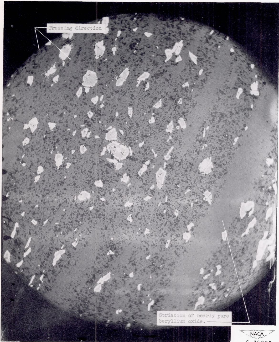
Figure 2. - Photomicrograph of 85-percent beryllium oxide plus 15-percent columbium showing coalesced metallic phase. X250.
