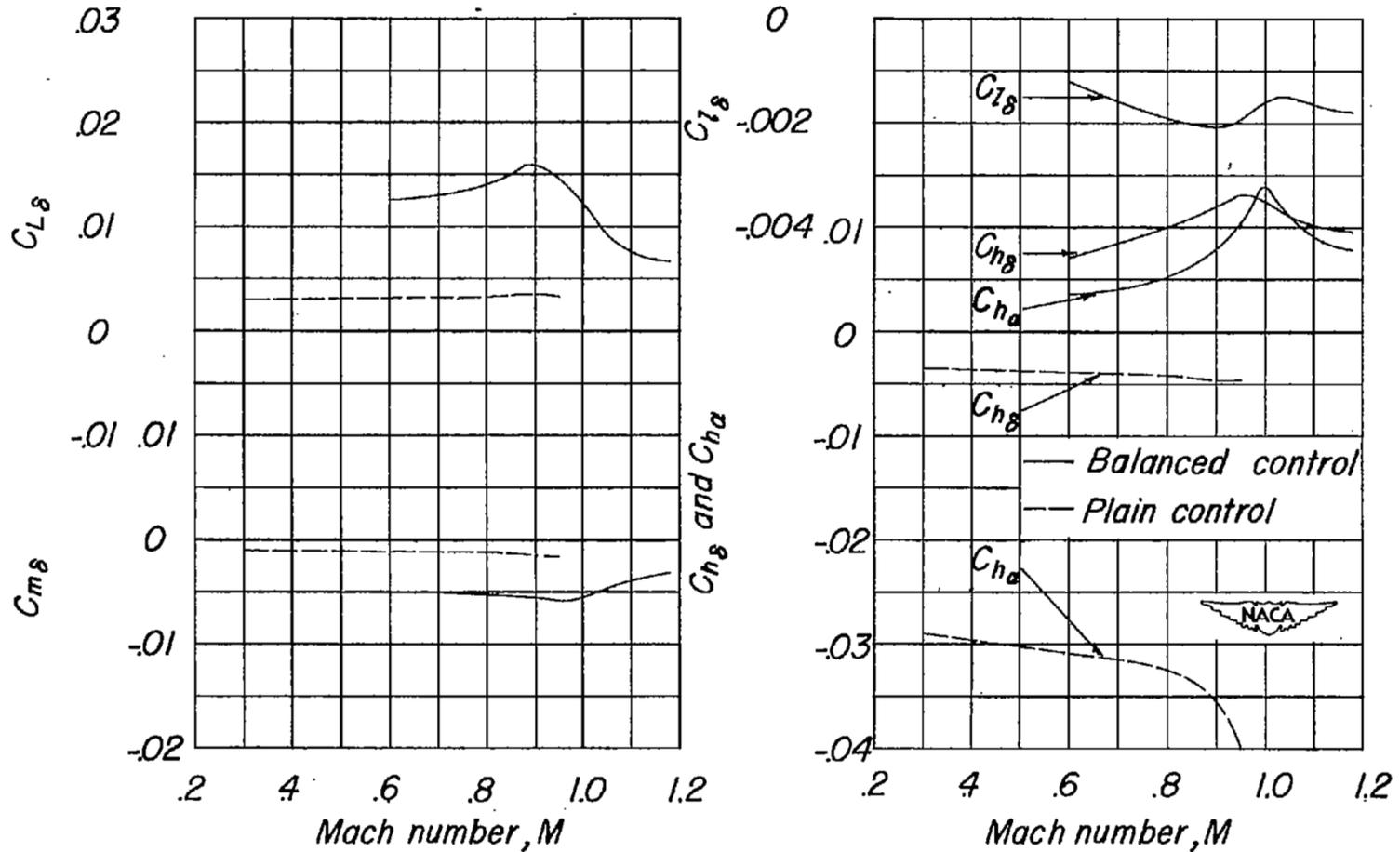
Figure 15.— The variation of the control parameters  $C_{L\delta}$ ,  $C_{m\delta}$ ,  $C_{l\delta}$ ,  $C_{h\delta}$ , and  $C_{h\alpha}$  with Mach number for a triangular control with overhang balance and a plain triangular control on a delta wing.  $\alpha = 0^\circ$  and  $\delta = 0^\circ$
