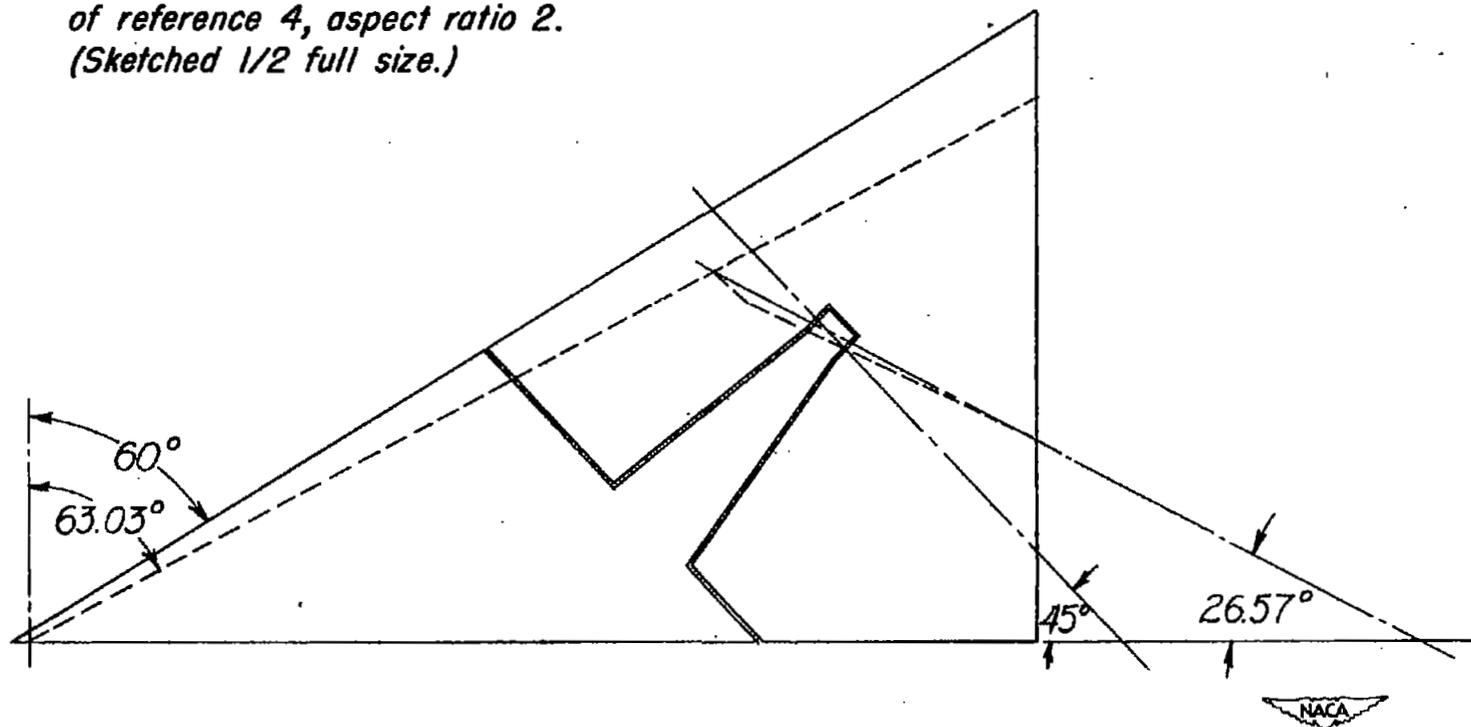
Figure 13.— Comparative sketches of general arrangements of the delta wing with balanced triangular control and delta wing with unbalanced triangular control of reference 4.
