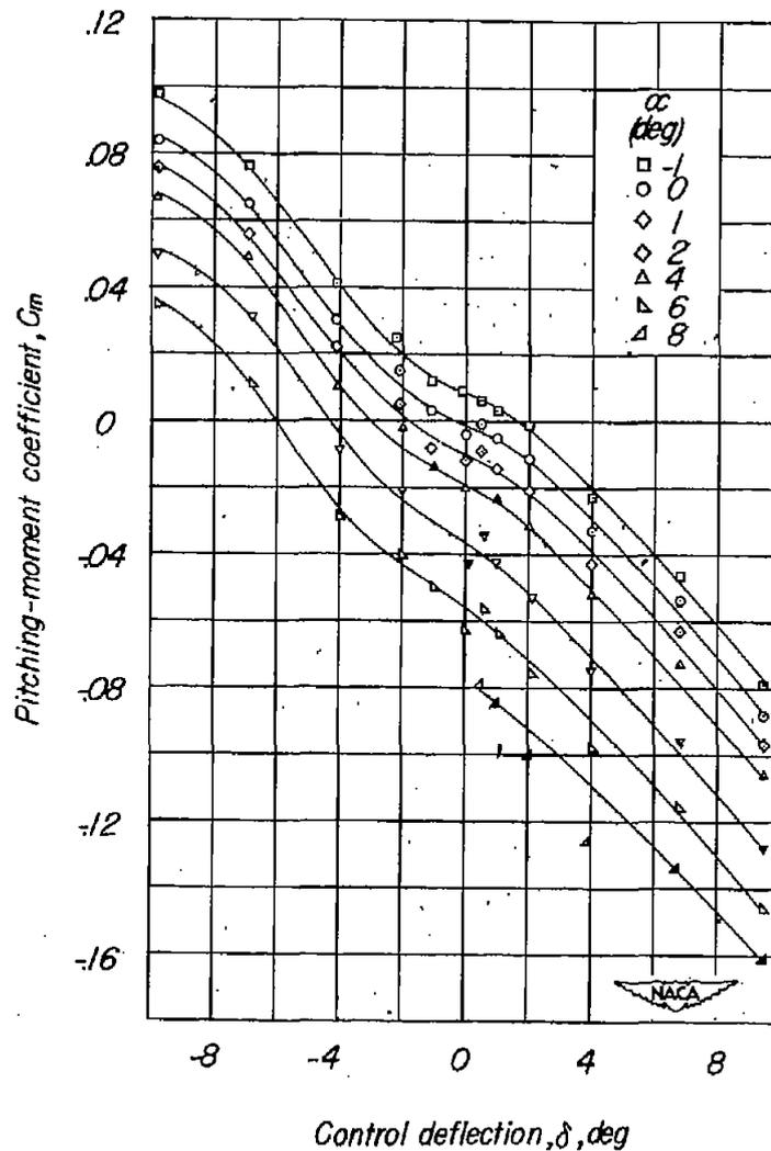
Figure 9.—Aerodynamic characteristics of model of  $60^\circ$  delta wing with triangular flap and overhang balance, aspect ratio 2.31, taper ratio 0, and NACA 65-006 airfoil.  $M=1.05$ .
