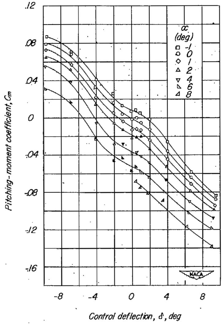
Figure 7.—Aerodynamic characteristics of model of  $60^\circ$  delta wing with triangular flap and overhang balance, aspect ratio 2.31, taper ratio 0, and NACA 65-006 airfoil.  $M=0.95$ .
