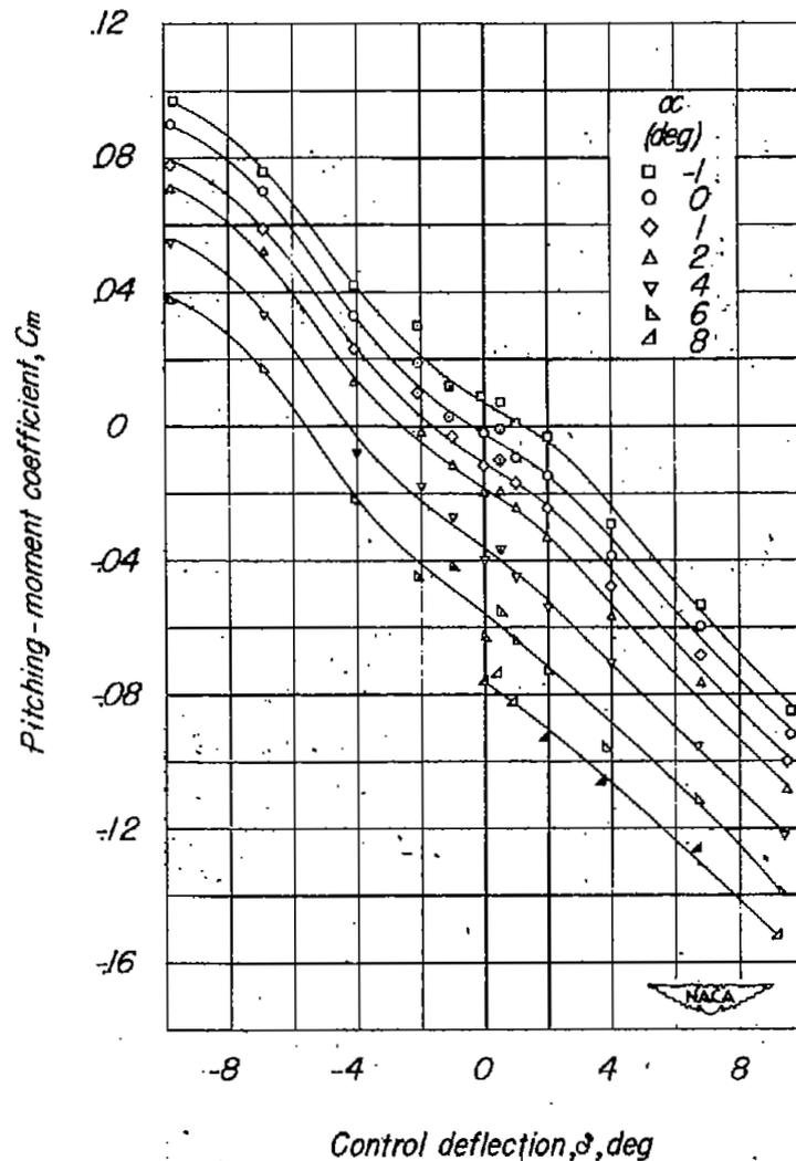
Figure 8.—Aerodynamic characteristics of model of  $60^\circ$  delta wing with triangular flap and overhang balance, aspect ratio 2.31, taper ratio 0, and NACA 65-006 airfoil.  $M=1.00$ .
