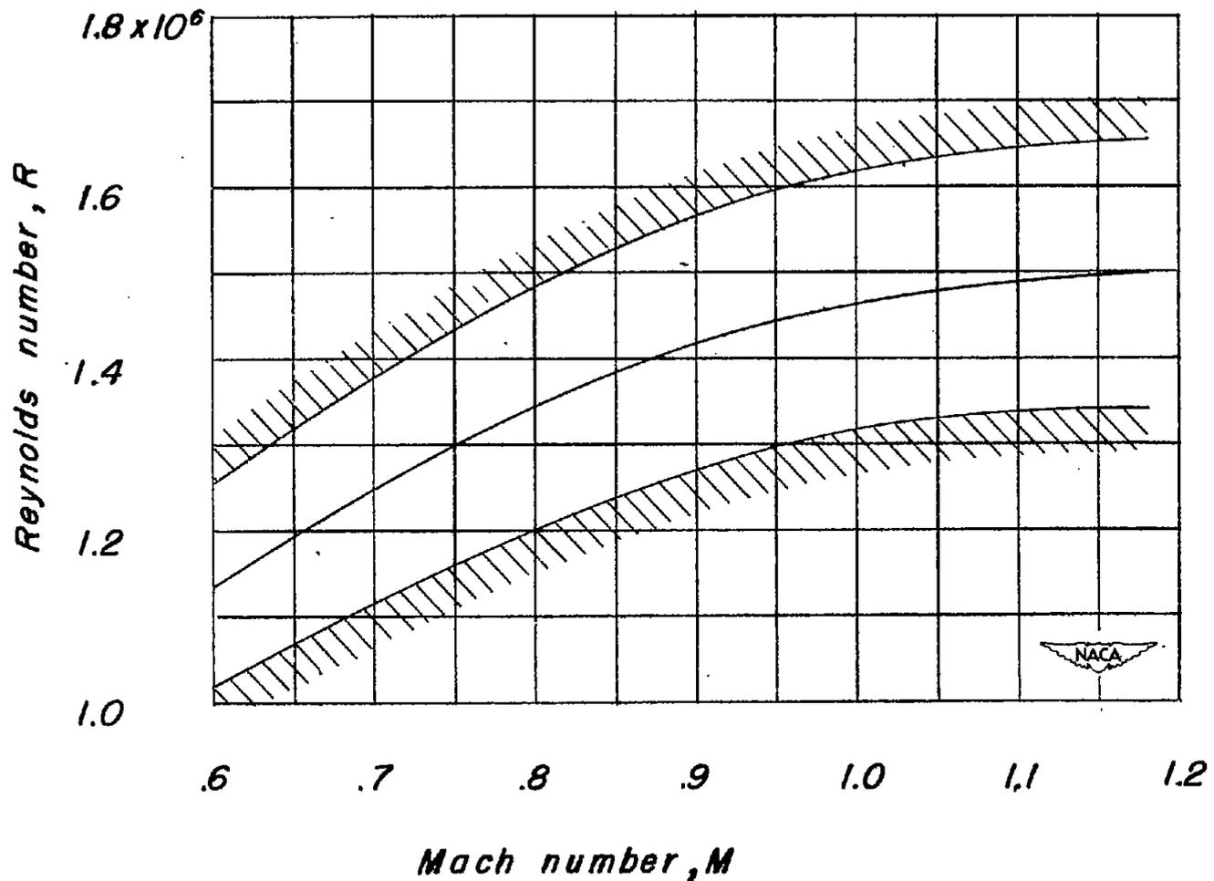
Figure 3.—Variation of test Reynolds number with Mach number for model of a 60° delta wing with triangular flap and overhang balance, aspect ratio 2.31, taper ratio 0, and NACA 65-006 airfoil.
