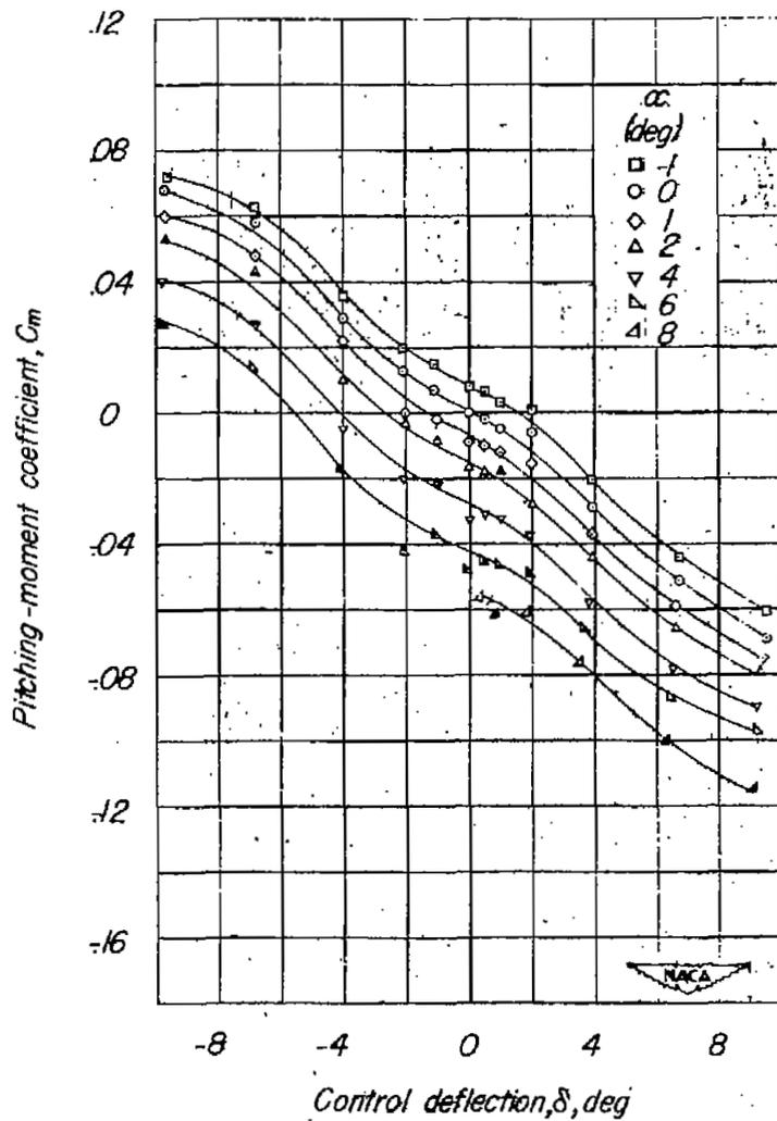
Figure 5.—Aerodynamic characteristics of model of 60° delta wing with triangular flap and overhang balance, aspect ratio 2.31, taper ratio 0, and NACA 65-006 airfoil.  $M=0.8$ .
