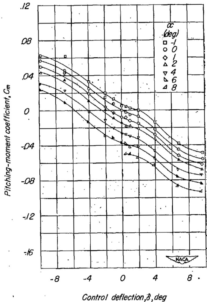
Figure 4.—Aerodynamic characteristics of model of  $60^\circ$  delta wing with triangular flap and overhang balance, aspect ratio 2.31, taper ratio 0, and NACA 65-006 airfoil.  $M=0.6$ .
