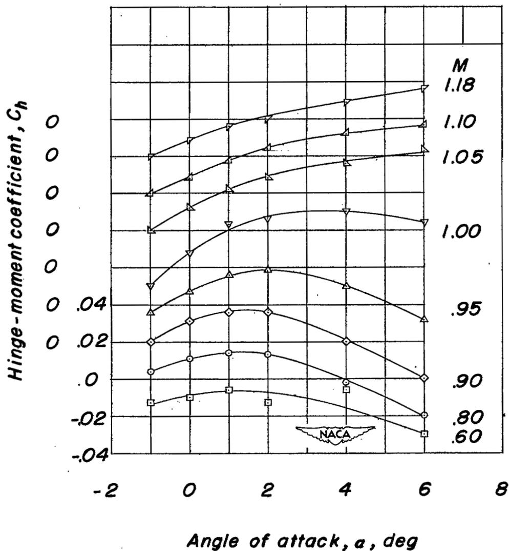
Figure 12.- The variation of hinge-moment coefficient with angle of attack for various Mach numbers.  $\delta = 0^\circ$ .
