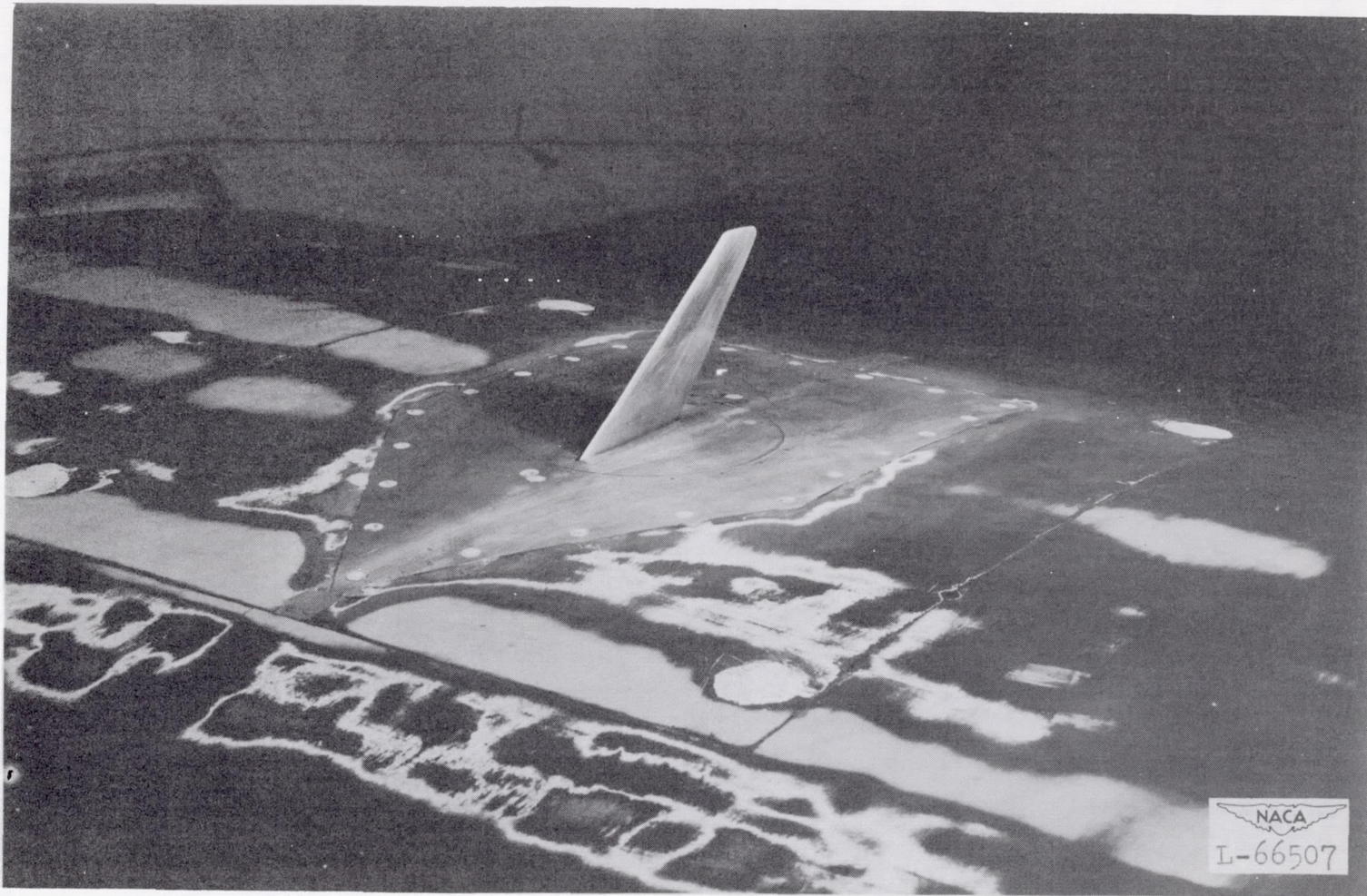
Figure 2.- Photograph of a model on the modified transonic bump.
