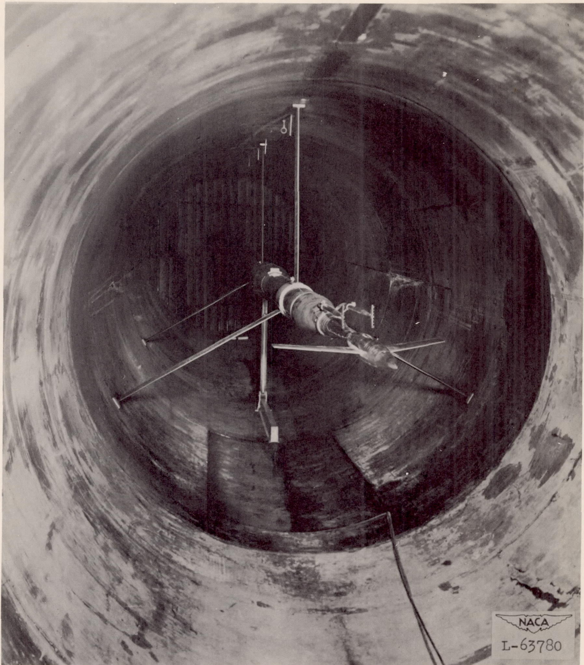
Figure 1.- Method of model installation in Langley 8-foot high-speed tunnel for present tests.
