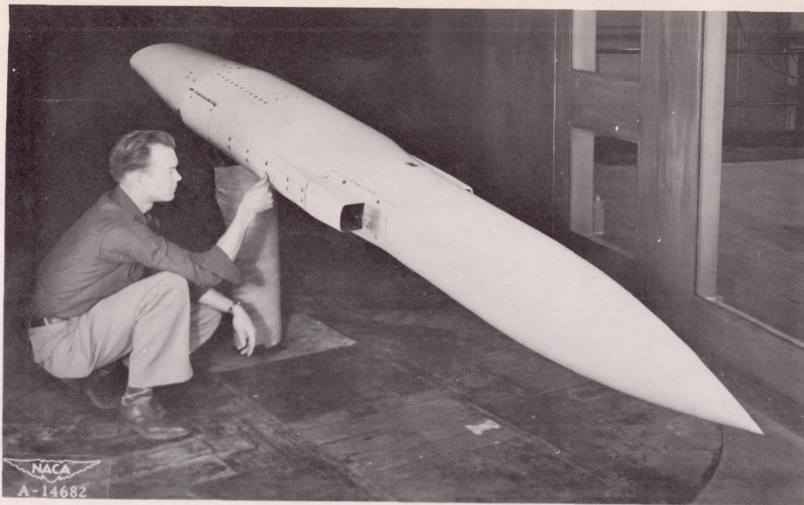
Figure 2.— The model rotated 90^{\circ} to permit testing at large angles of attack.
