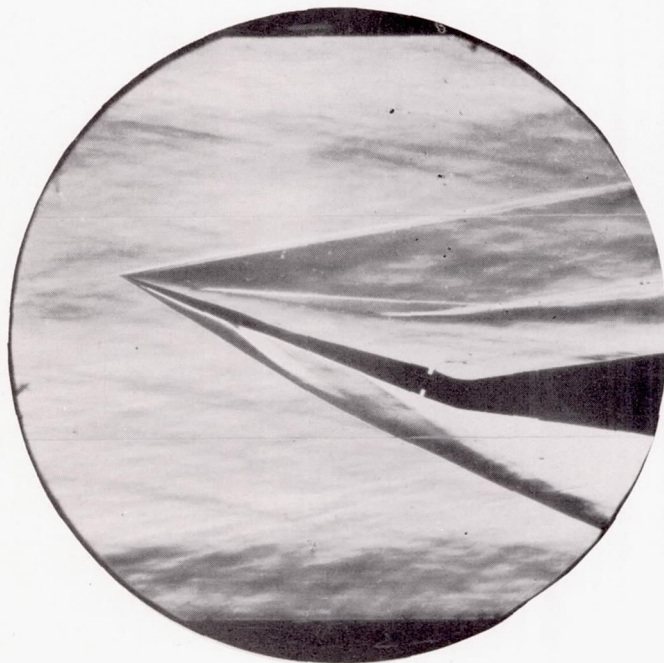
Figure 24.- Schlieren photograph of flow about a wing having a 5-percent-thick diamond section, \alpha = 16.8^\circ .
