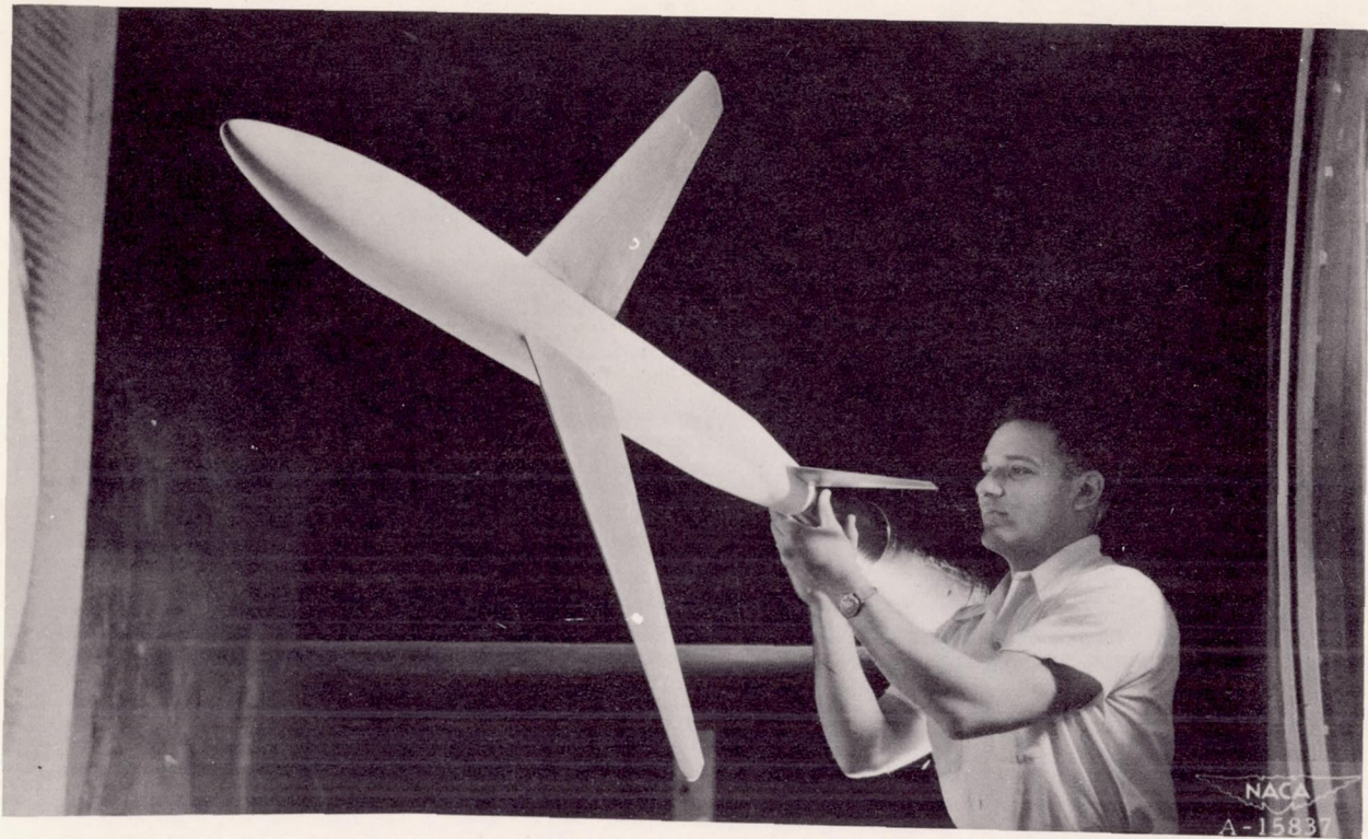
Figure 1.- The 1/15-scale MX-775A model mounted in the Ames 6- by 6-foot supersonic wind tunnel.
