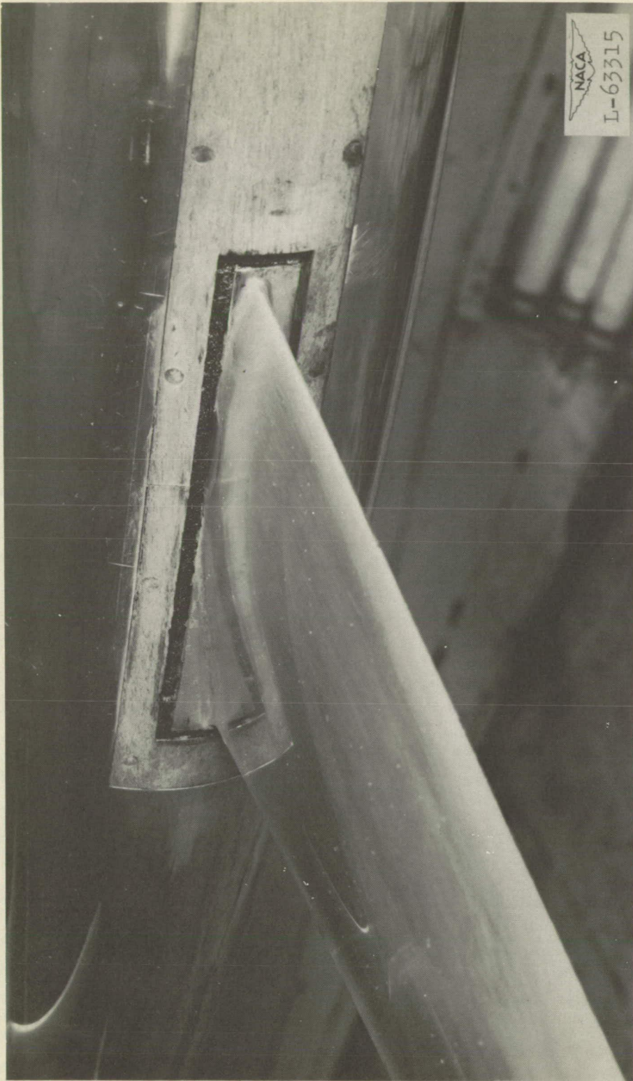
Figure 5.- Photograph of wing-fuselage juncture showing sponge seal.
