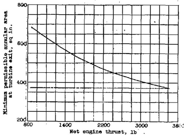
(c) Minimum permissible annular area at turbine exit.
