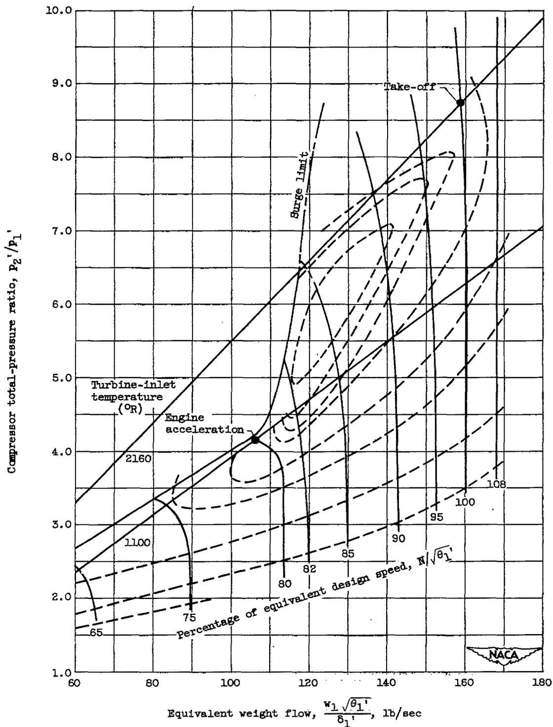
Figure 2. - Compressor map with lines of constant turbine-inlet temperature. Flight Mach number, 0; altitude, 0; no compressor-exit bleed.
