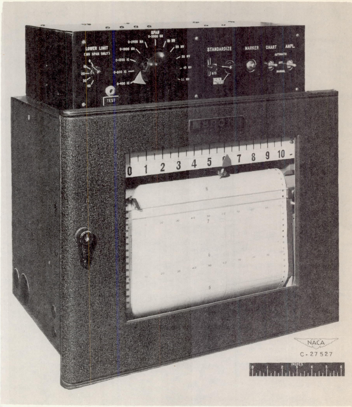
Figure 1. - Multiple-range self-balancing potentiometer.
