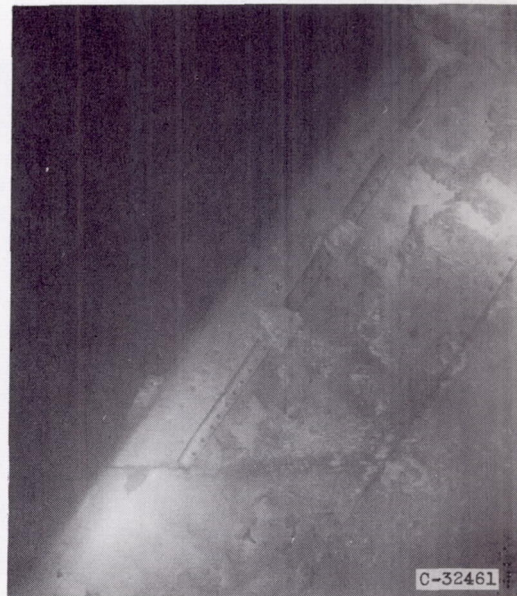
Lower surface. Icing time, 64 minutes; section drag coefficient, 0.0148.
