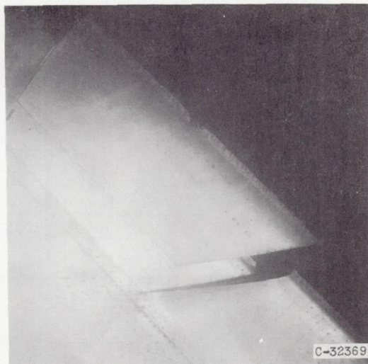
Upper surface. Icing time, 5\frac{1}{2} minutes; section drag coefficient, 0.0484.
