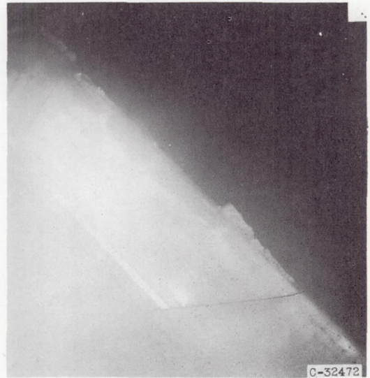
Upper surface. Icing time, 50\frac{1}{2} minutes; section drag coefficient, 0.0192.
