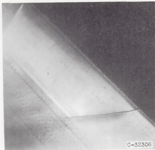
Upper surface. Icing time, 2\frac{1}{2} minutes; section drag coefficient, 0.0187.
