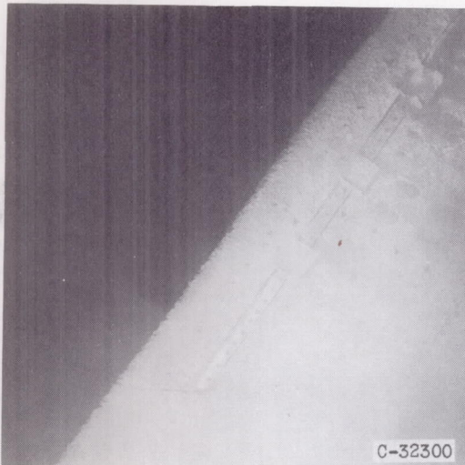
Lower surface. Icing time, 4 minutes; section drag coefficient, 0.0177.
