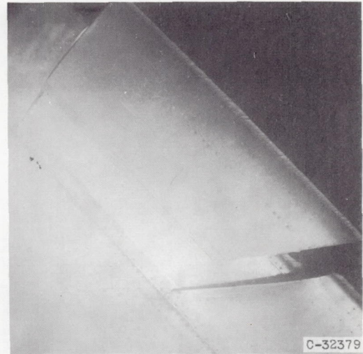
Upper surface. Icing time, 11\frac{1}{2} minutes; section drag coefficient, 0.0330.
