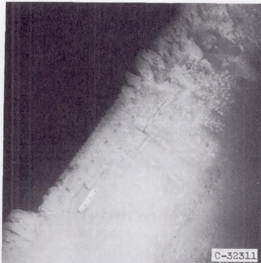
Lower surface. Icing time, 15 minutes; section drag coefficient, 0.0457.
