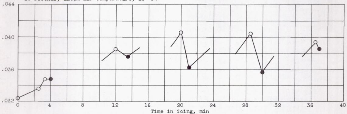
(c) Liquid-water content, 0.64 gram per cubic meter; heat-off period, 220 seconds; heat-on period, 20 seconds; datum air temperature, 10° F.
