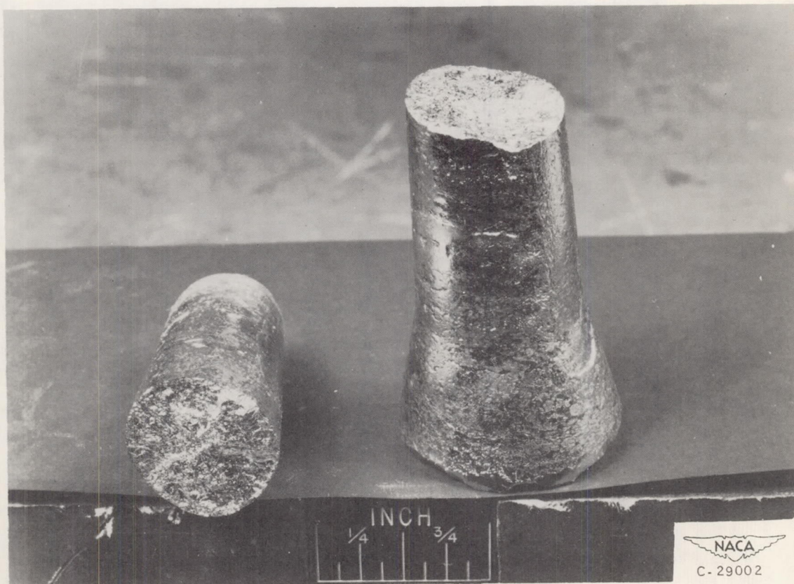
(b) Ingot cast in rammed zirconia mold.
