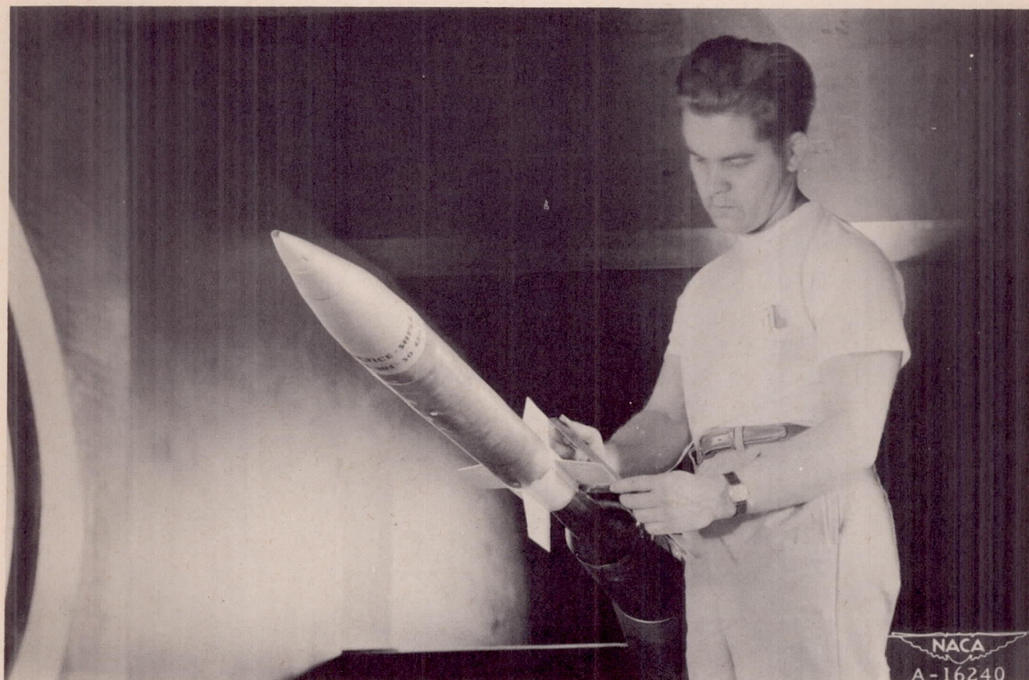
Figure 1.- Photograph of the 8-cm aircraft rocket mounted in the Ames 6- by 6-foot supersonic wind tunnel.
