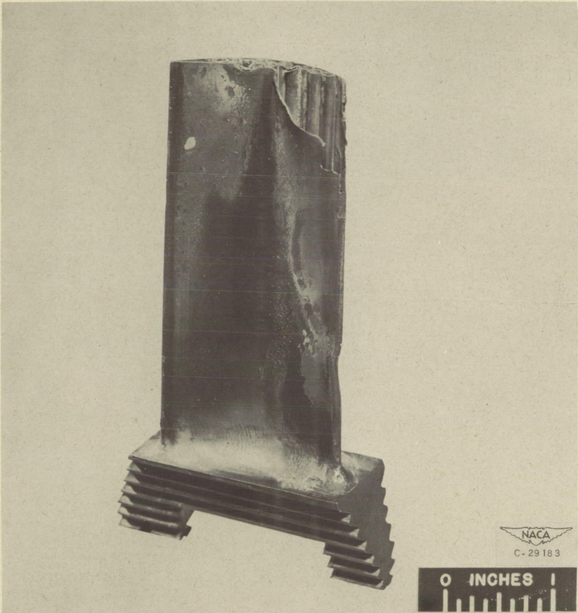
Figure 7. - Blade 14 after a total of 51\frac{1}{4} hours of rated-speed endurance test. Failure caused by vibration and erosion in area where there was poor brazing between tubes and shell.
