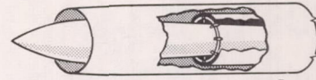
▽ Configuration C with 1\frac{1}{2} inch diameter sleeve; fuel injector 3\frac{5}{16} inches from outer wall.
