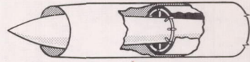
○ Configuration C with 1\frac{1}{2} inch diameter sleeve; fuel injector 2\frac{5}{16} inches from outer wall
