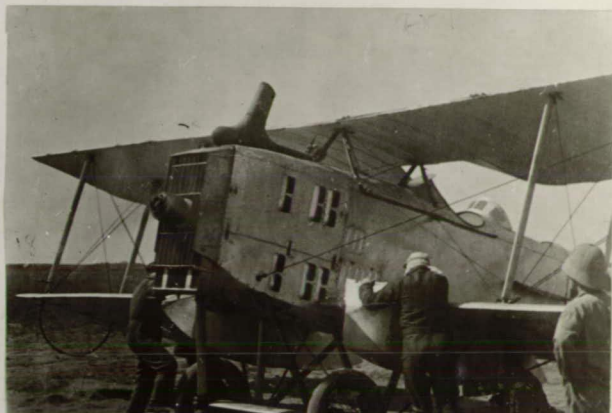
Erequet 14-t, standard airplane for Latecoere Line; at Alicante, Spain and Malaga. Note Streamlined containers for carrying air mail.
