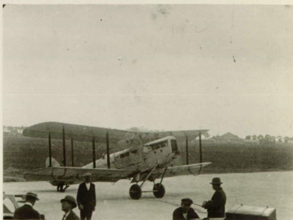
D.H.50 with Siddeley Puma 240 HP. engine, on cement mat at Paris Aerodrome; and being serviced at hanger rented from French Gov't by British air line.
