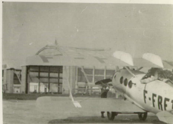
Installation at Strasbourg. Spad 46 with 400 HP. Lorraine-Dietrich engine. 12250 AS.
