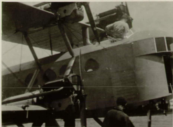
Eleriot passenger plane with 4 Hispano-Suiza 180 HP. engines, being tested at Le Bourget, Aug. 1934.
