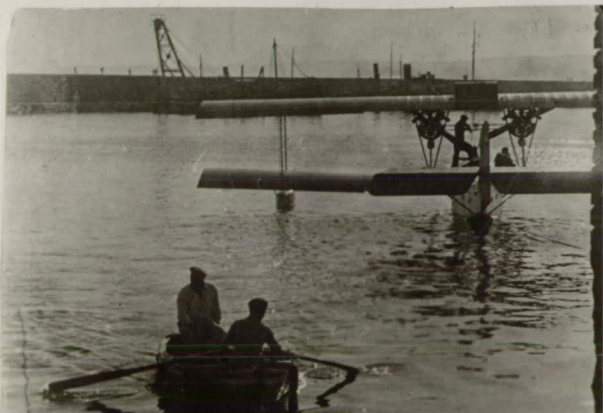
Liore and Olivier seaplane with two Hispano-Suiza 180 HP. engines, at Oran Algeria; used by Latecoere line between Alicante Spain and Oran.
