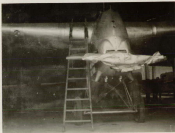
At Toulouse field, L.A.T. 16 monoplane with 400 HP. Lorraine-Dietrich engines, all metal.
