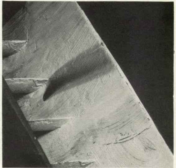
(b) Hydrogen sulfide introduced from tap in passage.
