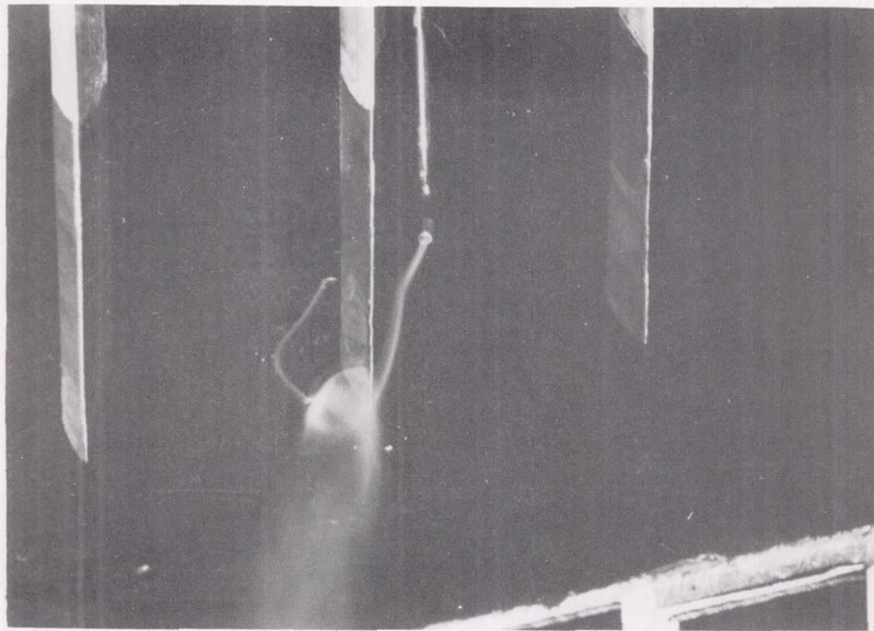
(c) Static tap near nose of blade and probe or wall near nose of blade. Stagger angle, 45^\circ .
