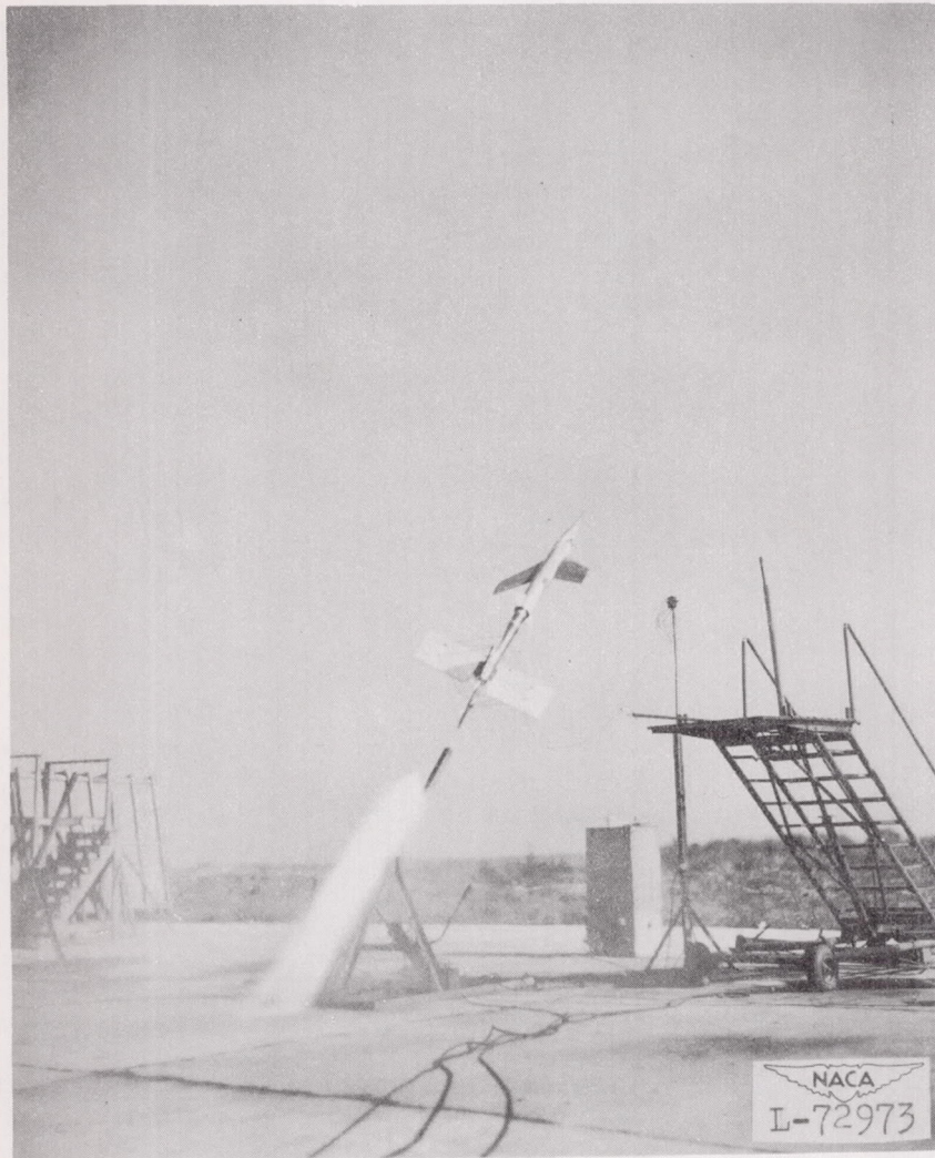
Figure 3.- Launching of a typical model-booster combination.
