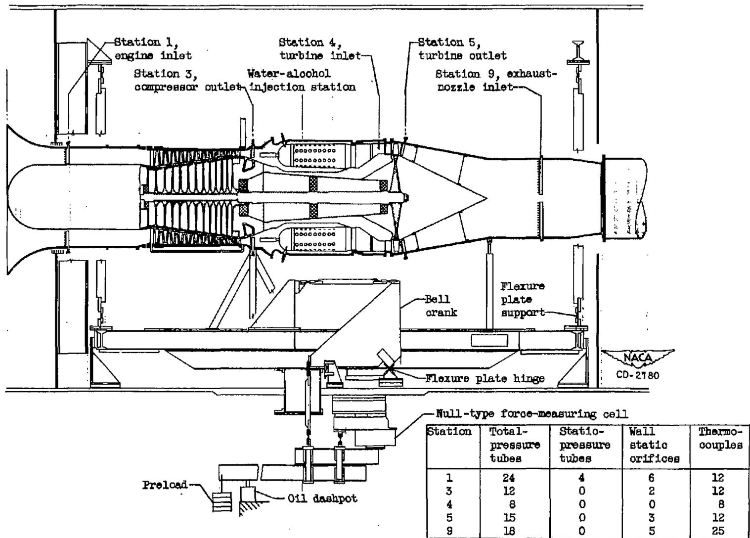
Figure 1. - Cross section of engine mounted in altitude test chamber showing location of instrumentation stations.
