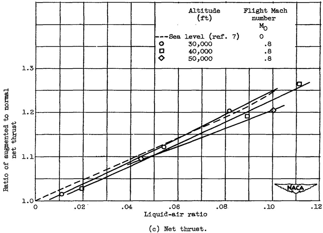
Figure 14. - Concluded. Effect of liquid-air ratio on exhaust-nozzle area and jet and net thrusts with engine operating at limiting turbine-outlet temperature of 1250° F. Engine speed for augmented operation, 7950 rpm; engine speed for normal operation determined by rated turbine-outlet temperature.
