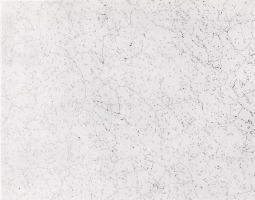
(a) General structure near leading edge showing heterogeneity in grain size and large number of carbides per unit of area. X250.
