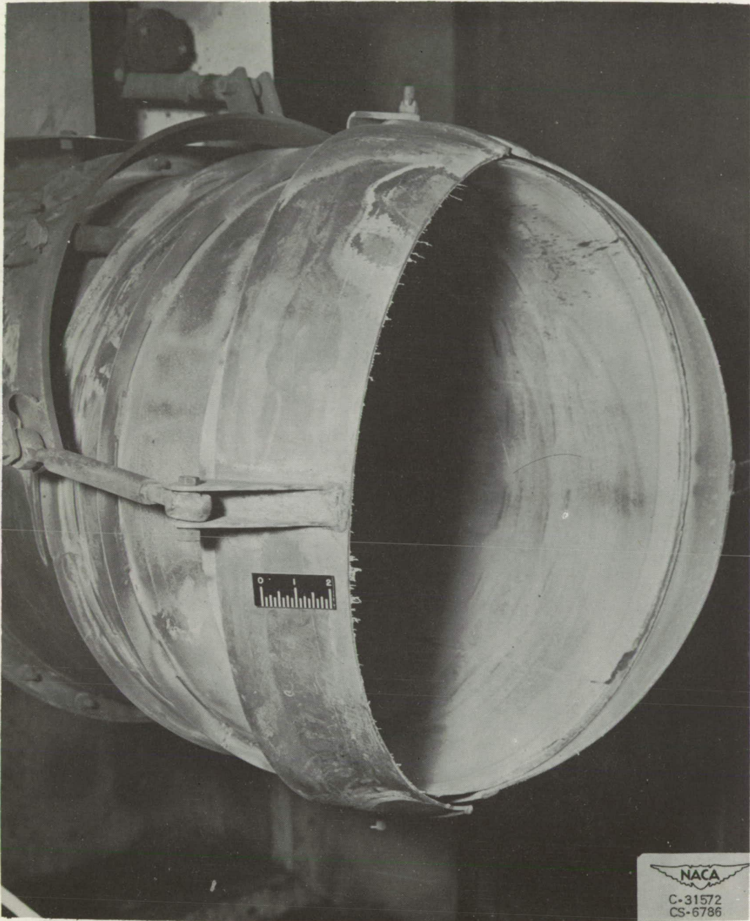
Figure 7. - Build-up of deposits on exhaust tail pipe nozzle.
