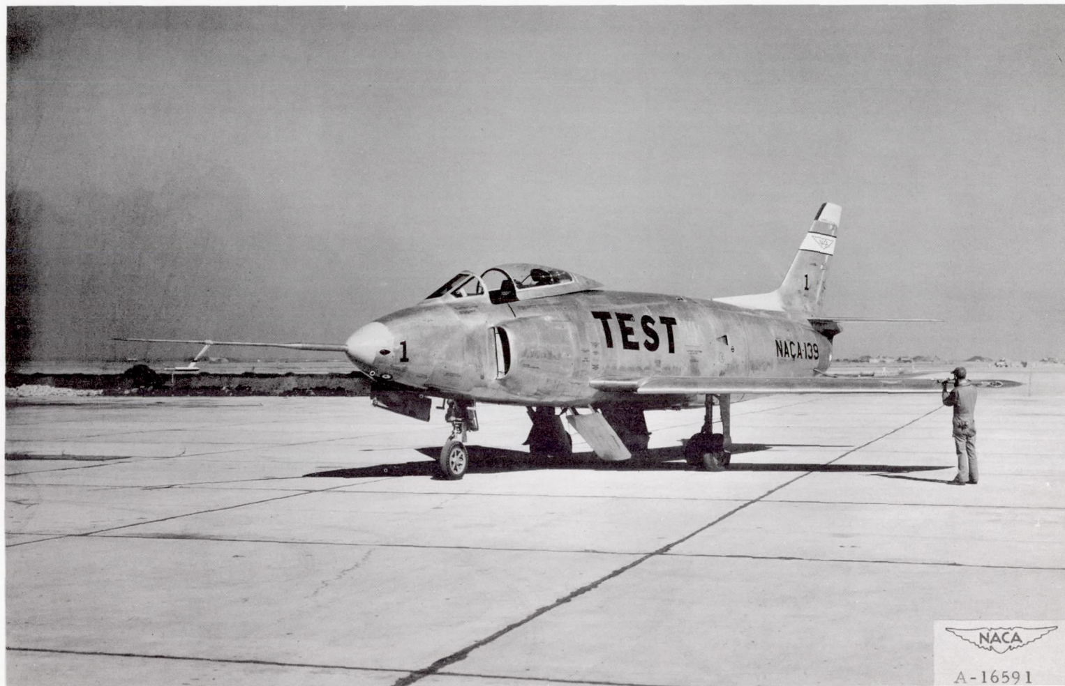
Figure 2.- The test airplane with ram-scoop inlets.
