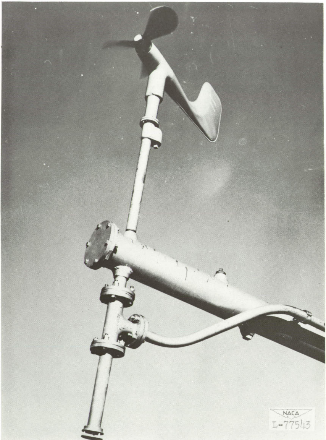
Figure 2.- Typical Aerovane installation on tower at Brookhaven National Laboratory.
