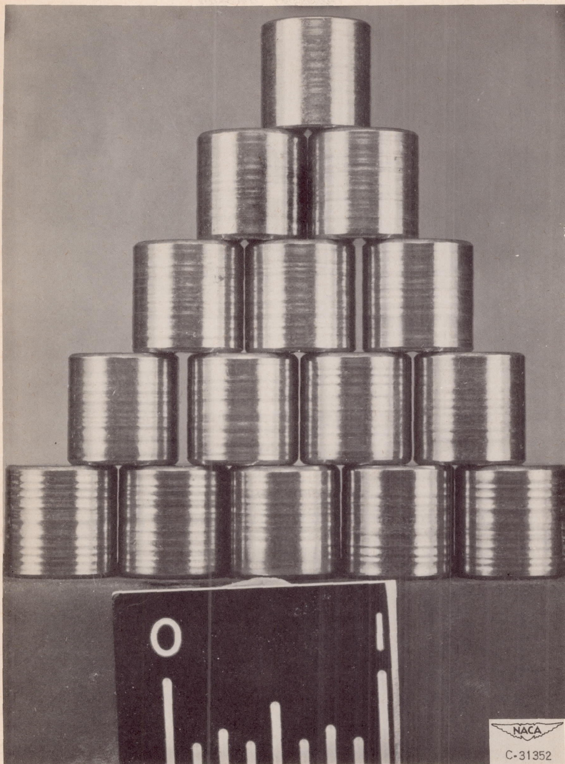
Figure 18. - "Wash board" roller wear of bearing 20 after test.
