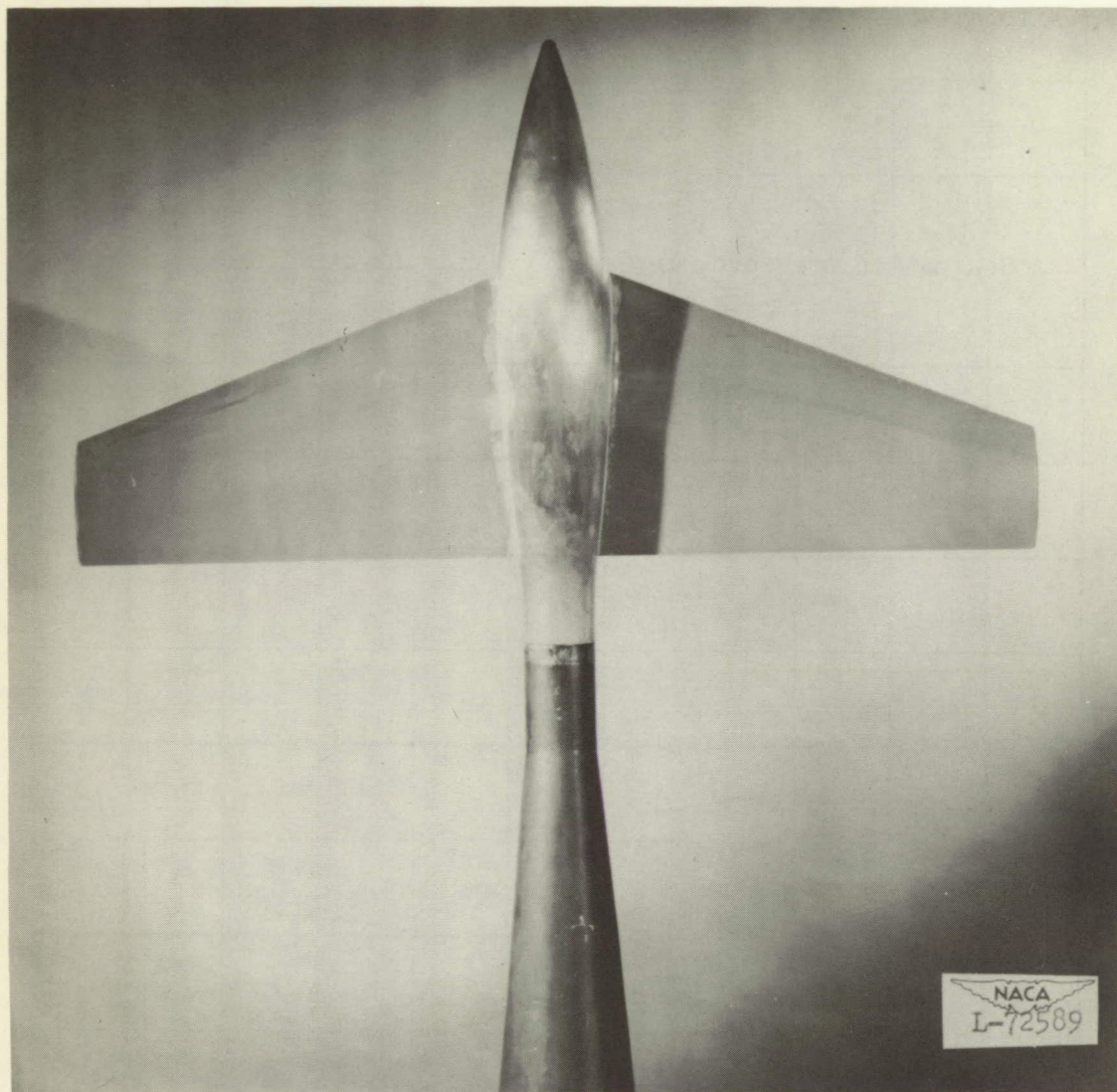
Figure 3.- Test model and conical balance fairing.
