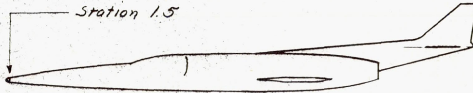
Nose Rounded at Station 1.5
