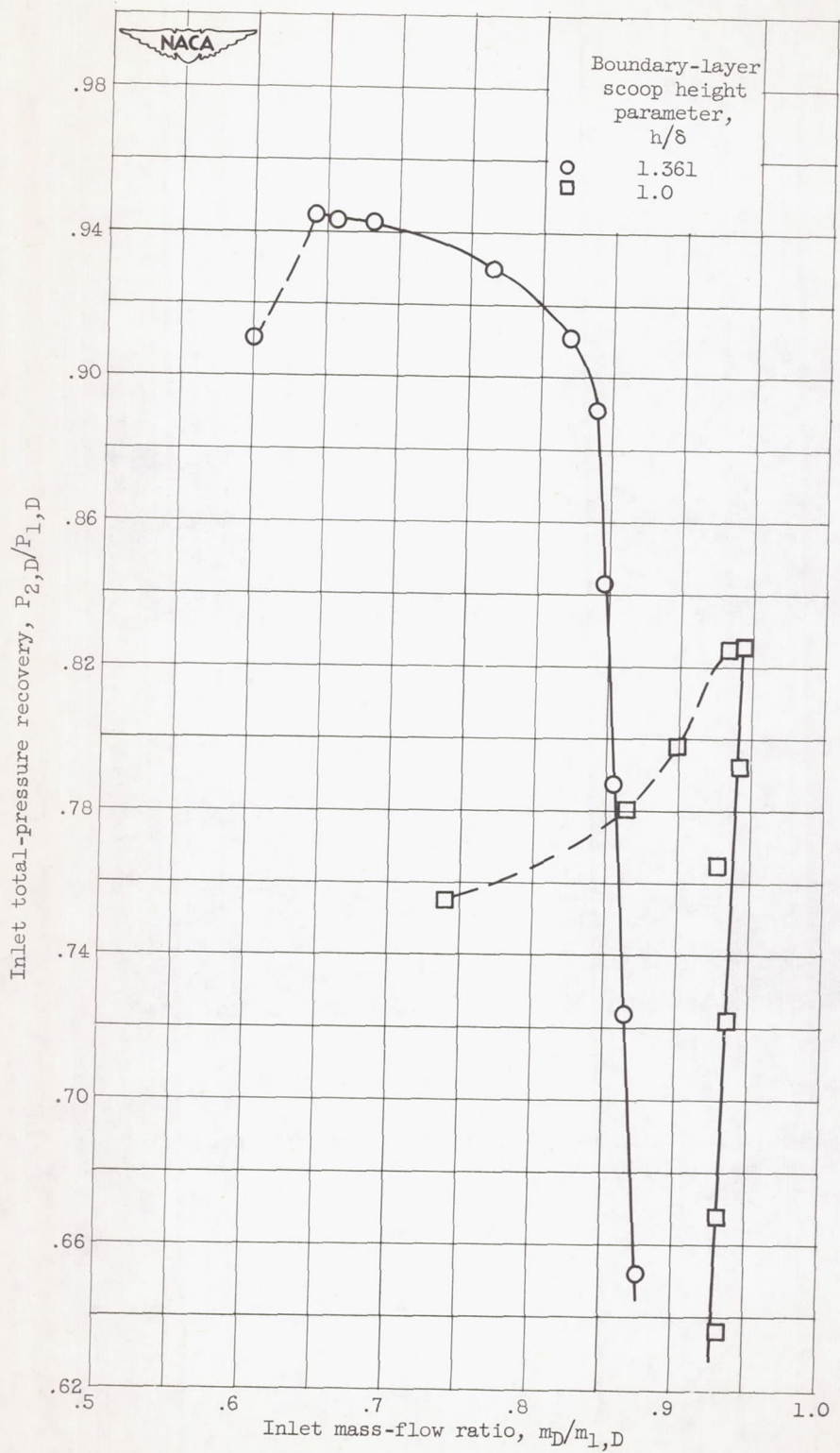
Figure 25. - Effect of cowl-lip scoop boundary-layer removal on inlet pressure recovery and mass flow at Mach 1.88.
